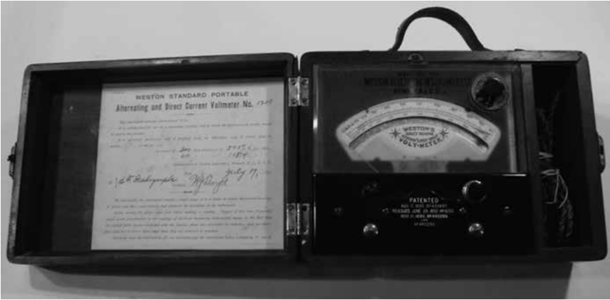
Fig. 10. Early Standard Meter last calibrated in 1895.
