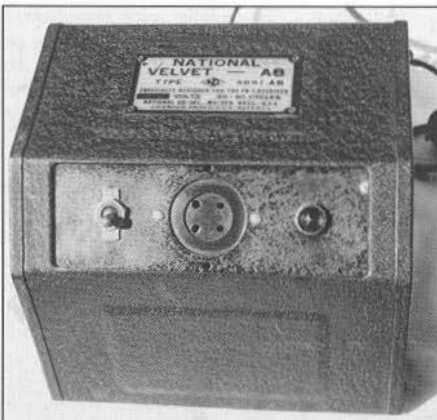
The 5897 Velvet AB supply, designed for the FB-7. Nameplate announces "ESPECIALLY DESIGNED FOR THE FB-7 RECEIVER." This particular unit was shipped with an early HRO.
