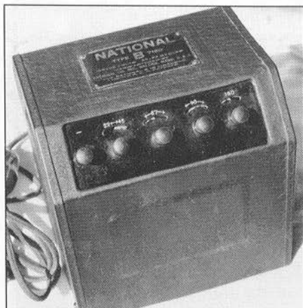
National 7180 B-eliminator. The four voltages are set by rockers above the terminals.
