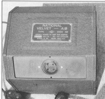
The 5880 Velvet AB supply, as used with the early Thrill Box receiver. Nameplate proclaims "ESPECIALLY DESIGNED FOR SHORT WAVE RECEPTION."
