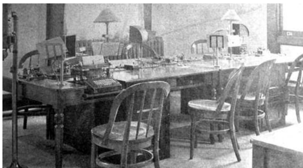
A Postal Telegraph "Octet" operator's table containing eight closets for storing a telegrapher's typewriter (four on each side).
