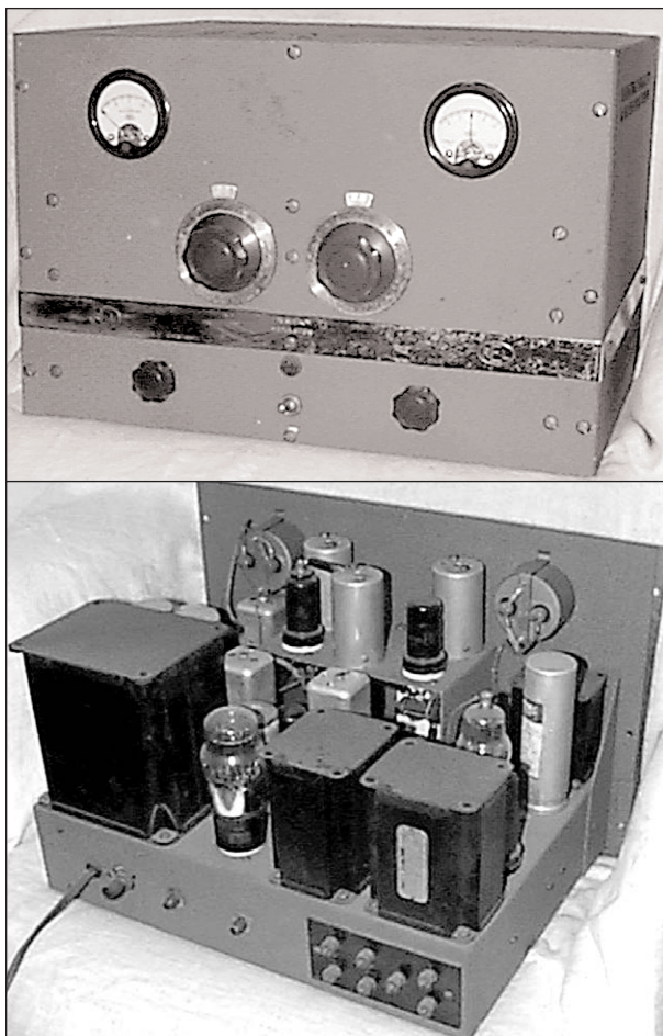
Front and interior views of the REL Model 517 receiver.
