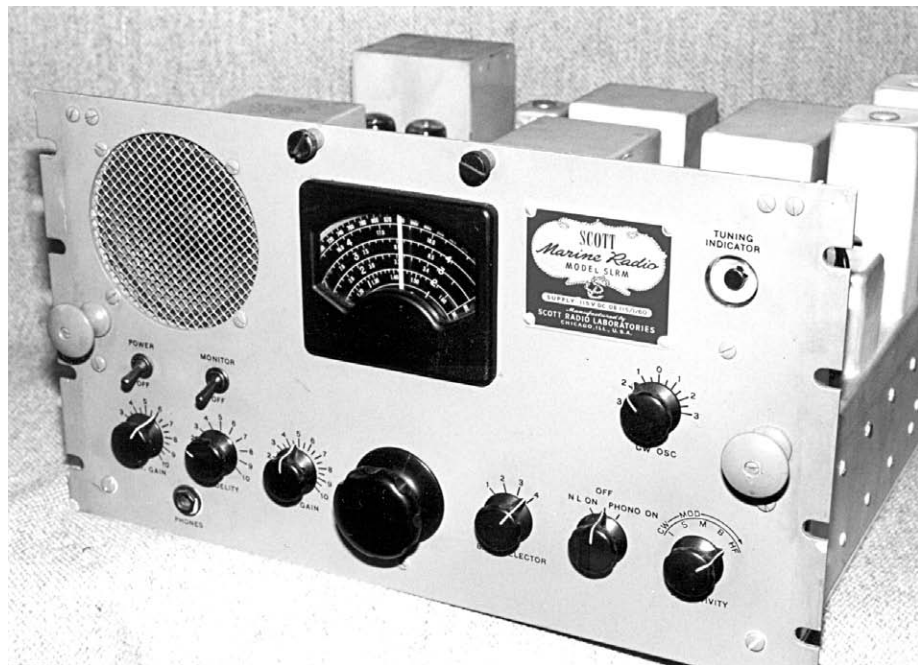
The SLR-M removed from the cabinet. Note the monitor speaker, the tuning eye tube, and the massive main dial.
