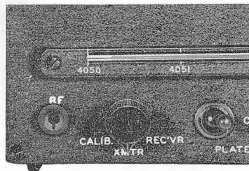
Selector switch on the Type 105-B MFM. The 103-B instrument does not have the CALIB. position for the switch.
