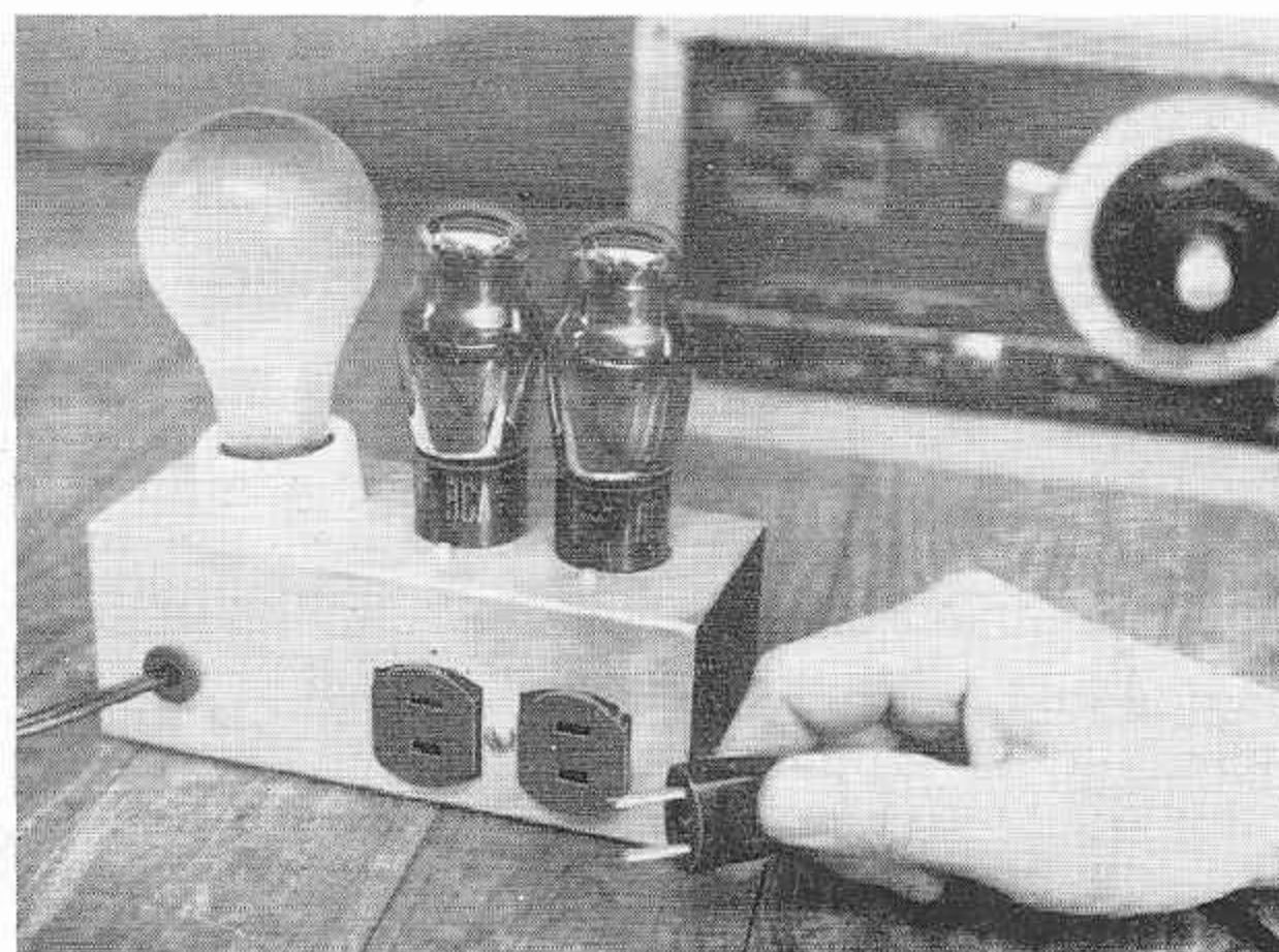
A simple, effective line-voltage regulator for the MFM, made from one 60-watt lamp and two VR-105 tubes.
