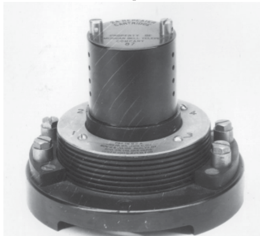
Fig. 3. 2-A production "repeater cartridge," 1910. Source: Bell Labs, courtesy Jerry Vanicek.
