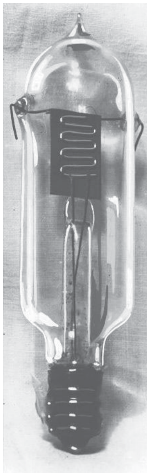
Fig. 12. First form of the gridded Audion, possibly the version that was in test in Dec. 1906. Source: ultimately unknown, but this retouched print is from De Forest Radio Co. files, ca. 1931.
