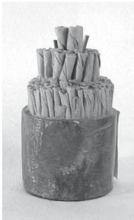
Fig. 14. A slice of the New York - New Haven "B" cable, placed in 1914 to reinforce the New York - Boston route. Wires are insulated with paper strip. Composition is seven quads of No. 10, 18 quads of No. 13, six pairs of No. 13, and 18 pairs of No. 16. Circuit capacity with phantoming is 99 circuits. Sample courtesy Dan Harley.
