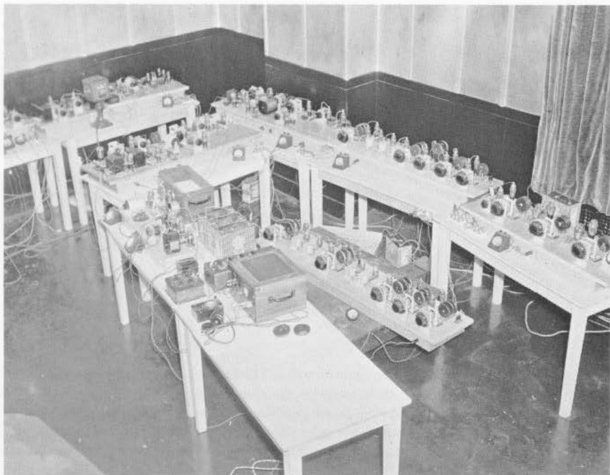
Fig. 2. Armstrong frequency modulation exciter equipment, used in the 1934-35 field tests, at the Empire State Building. The breadboard unit in the rear, just to the right of the microphone, was exhibited at a Canandaigua conference.
