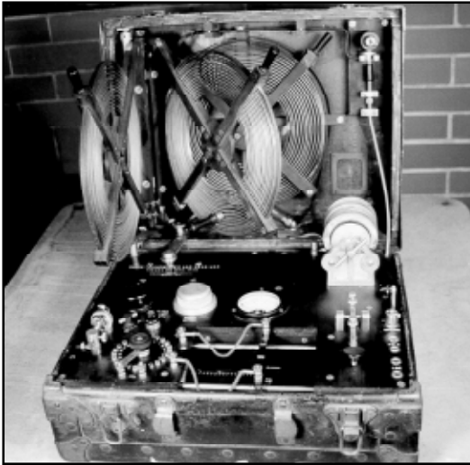
Figure 98. Wireless Specialty Apparatus Co. field set. Note quenched gap at upper right on panel. The key is on the lower right of the panel.
