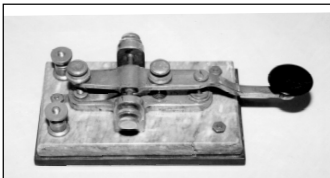
Figure 74. Wm. J. Murdock 2-kW key on marble base with heavy nickel-plated lever. The price was $8.00 in 1910.
