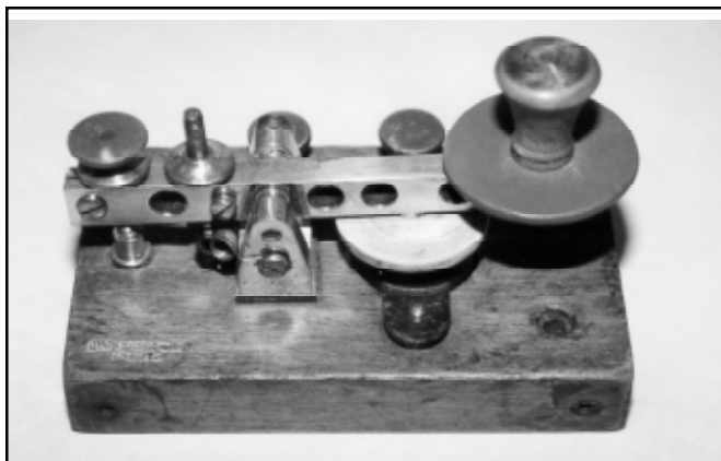
Figure 84. Ducretet and Roger of Paris, France. Oil break key made for aircraft use.
