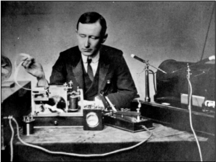
Figure 4. The Marconi Grasshopper key. There was no spring. The weight of the lever arm pulled the key down.
