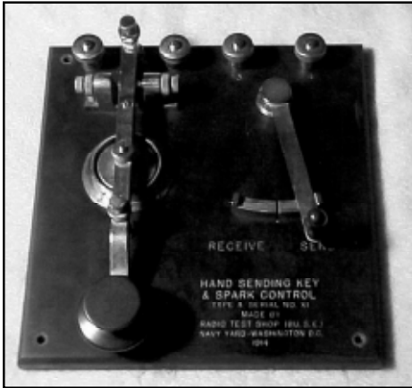
Figure 59. Washington Navy Yard, Hand Sending Key and Spark Control, 1914. The key is of the diaphragm type.
