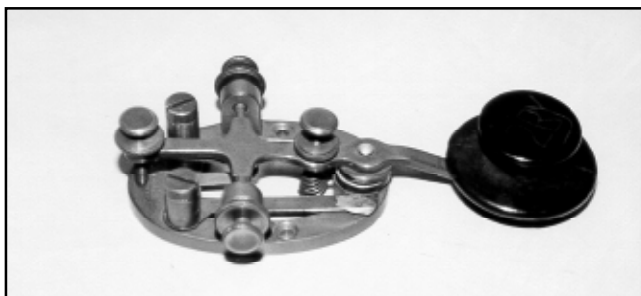
Figure 66. J.H. Bunnell key modified for heavier current capacity by adding large contacts. This key was used by station 2BY in Schenectady, NY, operating with 990-Watts on spark in 1922.
