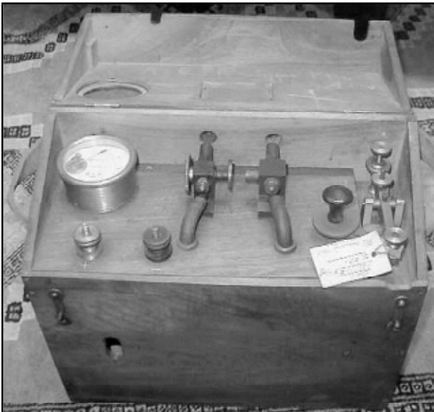
Figure 111. Radiguet and Massiot, Paris, France. Type 4 spark set with folding key. Made in 1917.
