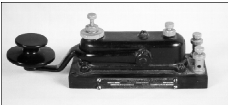
Figure 54. Wireless Specialty Apparatus Co., Type SE-653 for use with airplane sets. Rated at 4.5-amps at 150-volts.
