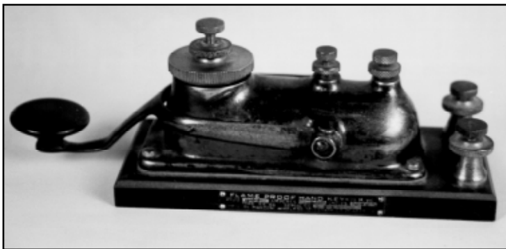
Figure 95. Marconi's Wireless Telegraph Company of America, SE-86 for use on submarines. Similar to the SE-144 by the Boston Yard.
