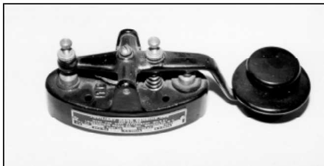
Figure 109. Lowenstein Radio Company, SE-923 for 1/4- and 1/2-kW transmitting sets. ca 1919.
