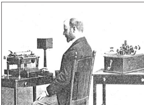
A telegrapher using his "mill" to copy messages played back on the embossed tape of the Phillips Morse Automatic Telegraph System instrument on the table at right.
