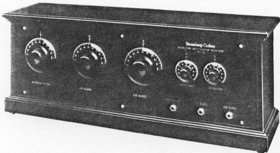
The first receiver manufactured by Stromberg-Carlson Model 1-A (1924). Neutrodyne circuit with 2 RF, Det. and 2 audio -- all 201-A's.
