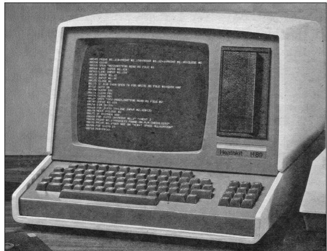
The H89 was only partly a kit. The CPU and terminal interface boards were preassembled, as was the keyboard and floppy disk drive. Assembly was limited to construction of the power supply, mounting the boards and plugging in some connectors. The H89 was also available without the computer board and disk drive, and sold as the H19 “smart terminal.”
