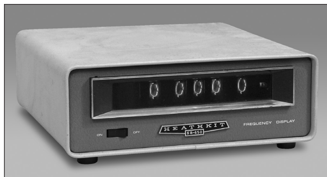
The Nixie tube-based SB-650 was the amateur group's first digital product.
