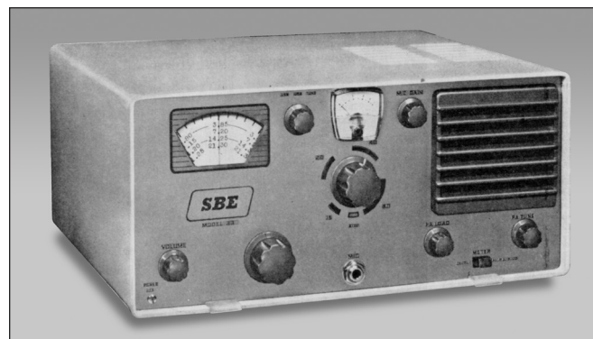
The Sideband Engineers SB-33, introduced in 1962, proved that solid-state transceivers were possible, practical, reliable—and affordable—years before most manufacturers made the leap to transistors. QST, December 1962.
