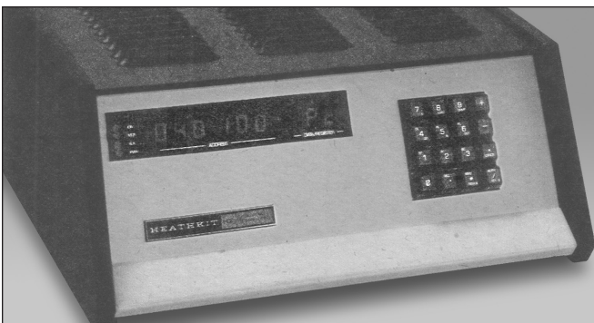
The H8 used Intel’s 8080A processor and was designed for the hobby user. It could be upgraded to as much as 64K of RAM. Who would ever need more than that?
