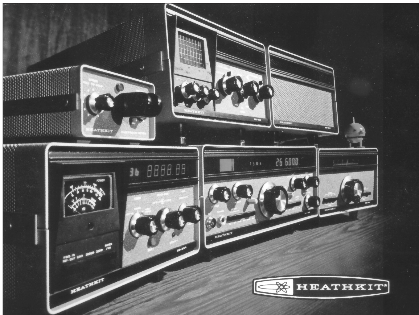
This image is from a QSL card Heath provided with the SB-104. It is oddly emblematic of the problem-prone rig—the time on the clock reads 88 88 88, and more to the point, the frequency shown reads 26.600 MHz.
