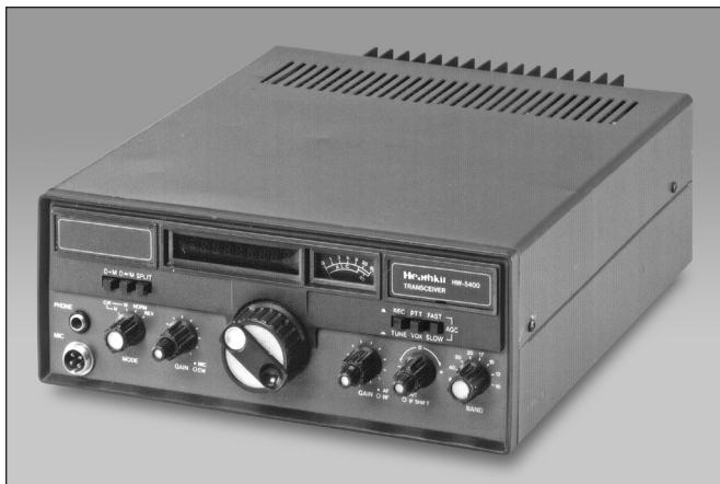
The HW-5400. Heath's last stand. Complicated and expensive. It lacked computer control, but included the WARC bands.
