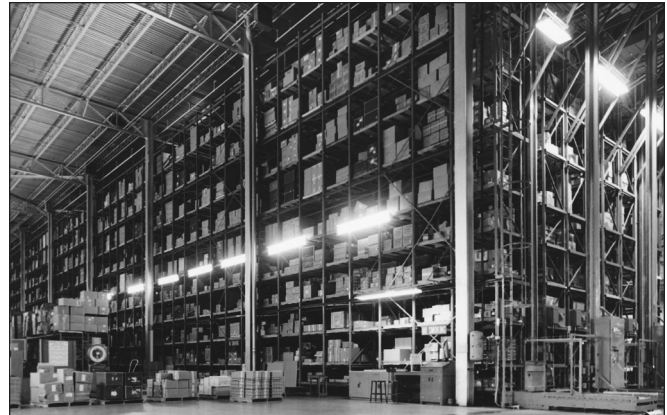
Heath's computerized "stacker," installed in 1967, was a kind of robotic fork-lift. It could efficiently store and retrieve inventory by means of punched cards.
