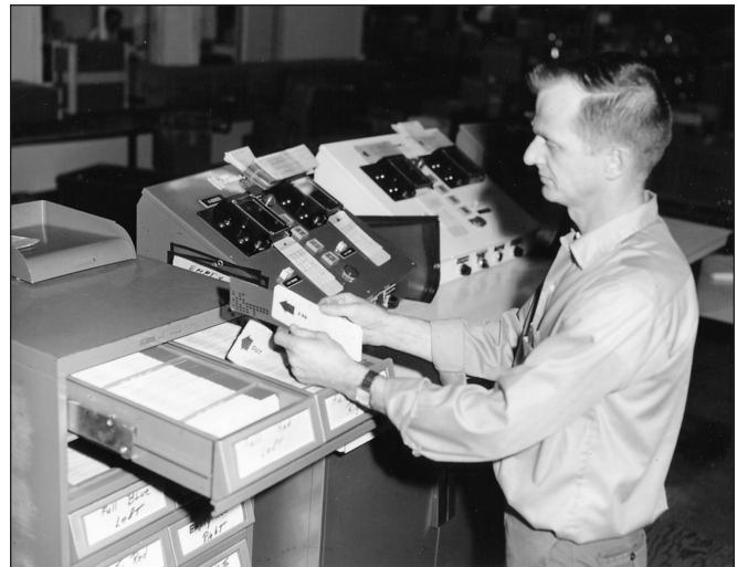
Using punched cards, a worker prepares to send the stacker on a mission. The cards contain the part or model number and location of the inventory to be retrieved.
