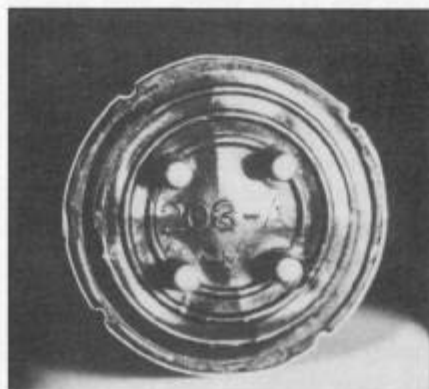
Molded marking on the base of a 203A/VT-1.
