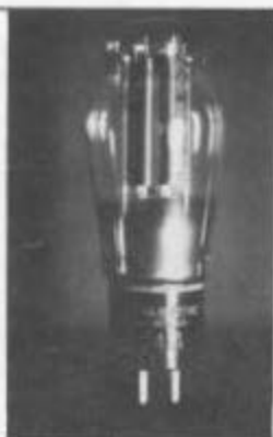
The 274A rectifier, probably the first WECO tube with an ST bulb.
