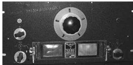
RAS-3 front panel—note coil locks.
