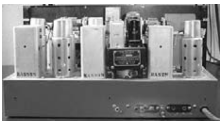
Rear of RAS—note plug-in noise limiter chassis.
