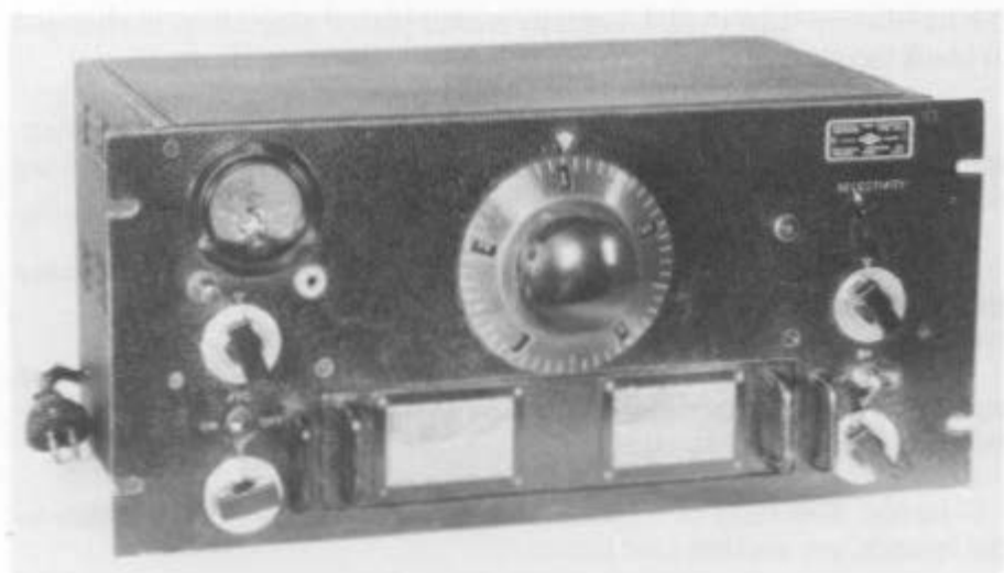
Fig. 3. Very late plug-in crystal HRO (169 L, about 1940). Note illuminated plastic-case meter and rectangular selectivity knob.
