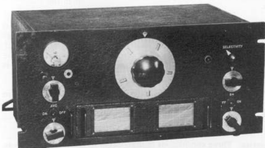
Fig. 2. Example of earliest HRO without white pushbutton, also showing engraved panel rack model (F 213, mid-1935).
