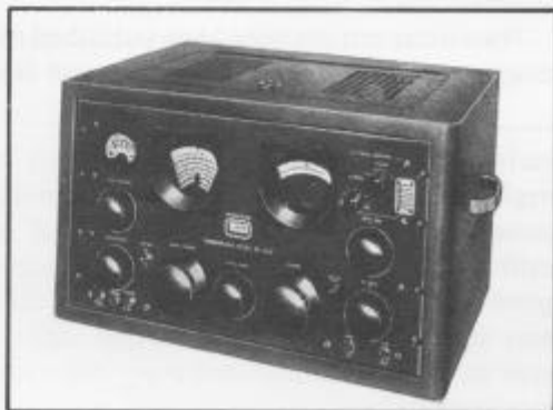
Fig. 8. The 1952 Super-Pro 600 20-tube, double conversion, high-performance receiver. This is the JX model.
