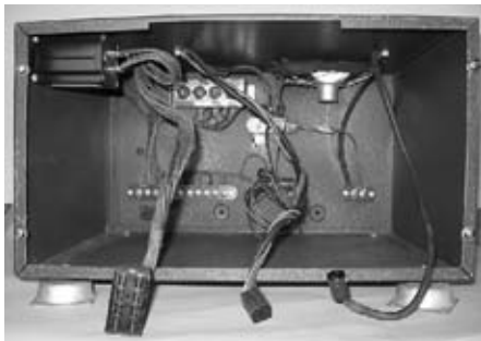
Cabinet Interior—Filament transformer at upper left (see text).
