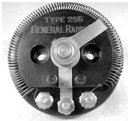
Fig. 2. The cleaned resistance wire back in place on the rheostat body.
