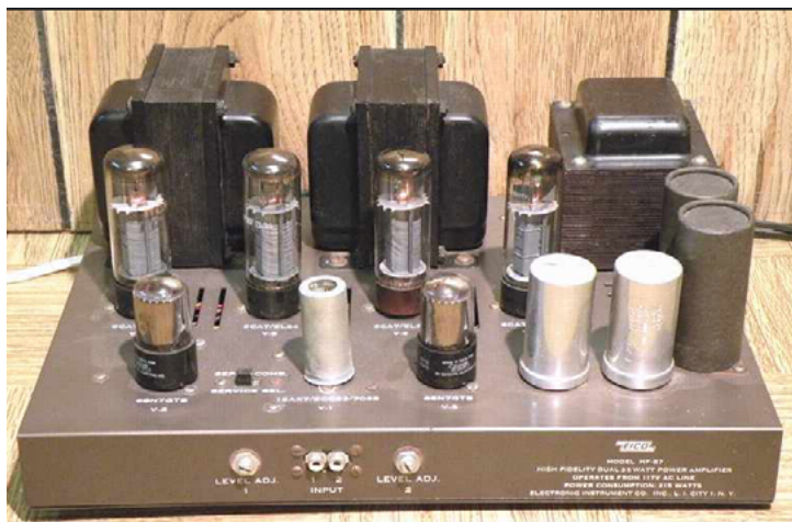
EICO model HF87 amp with four EL-34 output tubes and 70 watts RMS (35 watts per channel). (KB8TAD photo)
