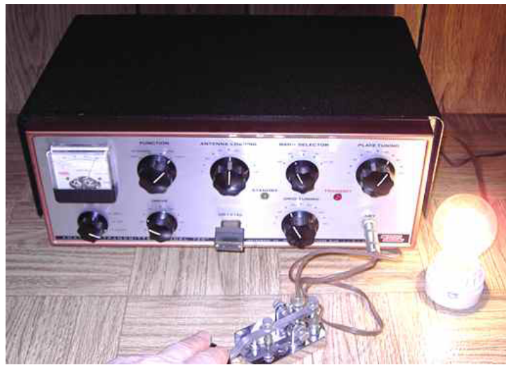
EICO 720 transmitter at 90 watts input and 60 watts output to dummy load bulb. (KB8TAD photo)
