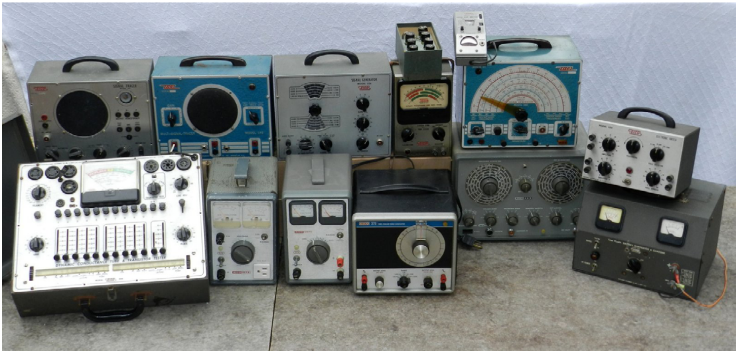
A gathering of EICO test equipment. Foreground from left, Model 666 Dynamic conductance tube and transistor tester, Model 1078 dual metered Variac, 1064S dual metered low voltage supply, 379 Sine/square wave generator, 369 Sweep generator, 1060 Low Ripple battery eliminator and charger, Top row from left, Model 147 signal tracer, 145 signal tracer, 324 RF Signal generator, 944 Flyback & yoke tester, 360 TV-FM Sweep generator, 488 Electronic Switch. On top, Model 710 Grid Dip meter and coils. (KB8TAD photo)
