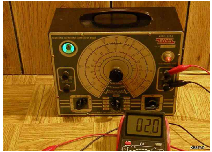
EICO 950A resistor-capacitor bridge testing the leakage and reforming neon indicator circuit at 2 mA. (KB8TAD photo)
