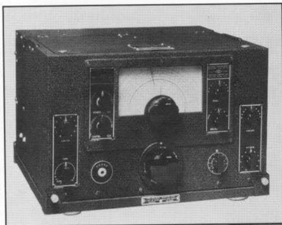
Figure 38. Model RAO-6 receiver in mounting rack. This is also designated an NC-120.
