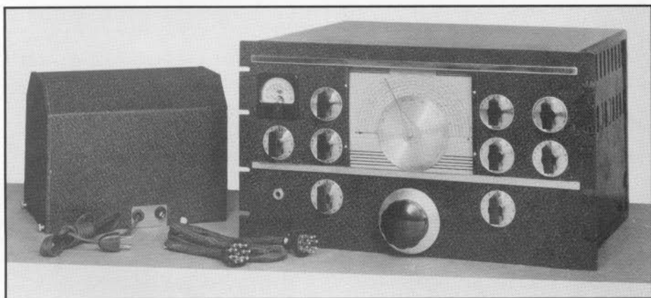
Figure 12. NC-2-40 receiver with external power pack. This is a developmental version, and it is doubtful that any reached the market.
