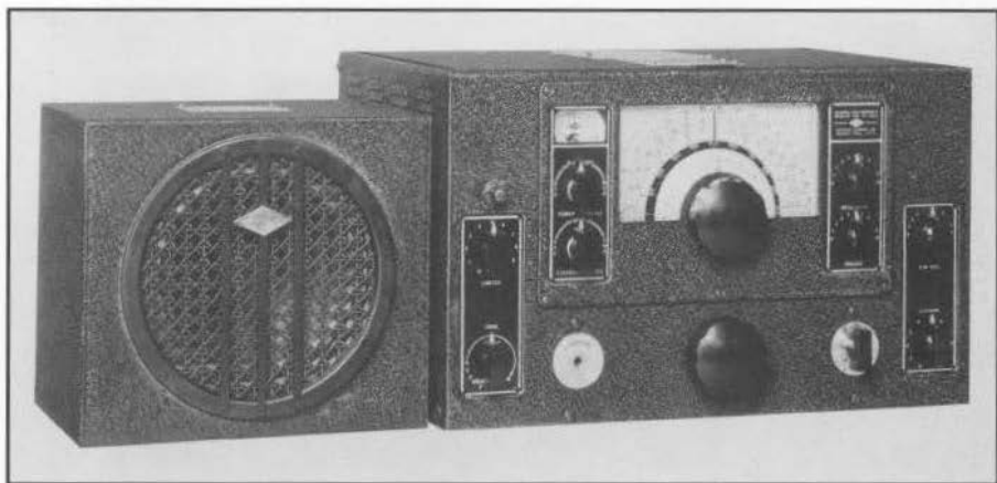
Figure 17. The RAO-1 equipment. This receiver, with the military labels on the top of each piece, is actually an NC-100XA.
