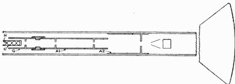
*Fig. 4. In the sketch of the RCA type 906 tube the following letters indicate the various elements: H, the heater; C, cathode; G, shield grid; A1, first anode; A2, second anode. The two pairs of deflecting plates are to the right of A2. It will be noted that these plates are at an angle to the main axis of the tube. This arrangement of elements in a glass envelope or bulb constitutes what is sometimes referred to as an "electron gun."*
