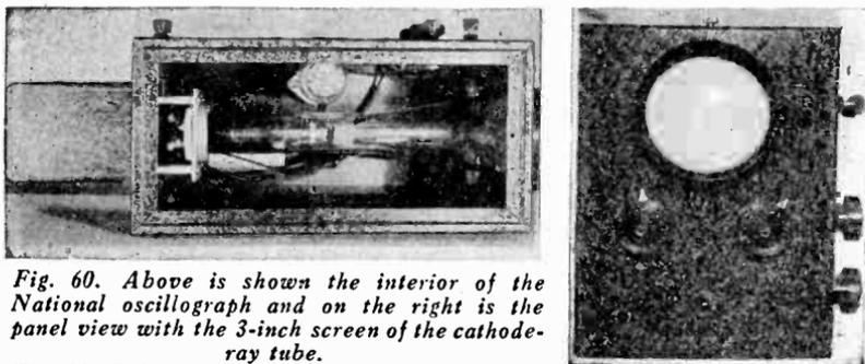
Fig. 60. Above is shown the interior of the National oscillograph and on the right is the panel view with the 3-inch screen of the cathode-ray tube.
