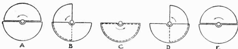
*Fig. 259. Five positions of the rotating plates of a variable condenser used in a frequency modulator. When the capacity is minimum (plates unmeshed completely), the frequency is maximum and vice versa. It is essential that the plates be in positions B or D when the oscillator delivers the mean frequency of the circuit under test.*
