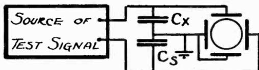
*Fig. 216. Circuit for comparing power factors or losses between two condensers.  $C_x$  is the sample and  $C_s$  is the standard.*
