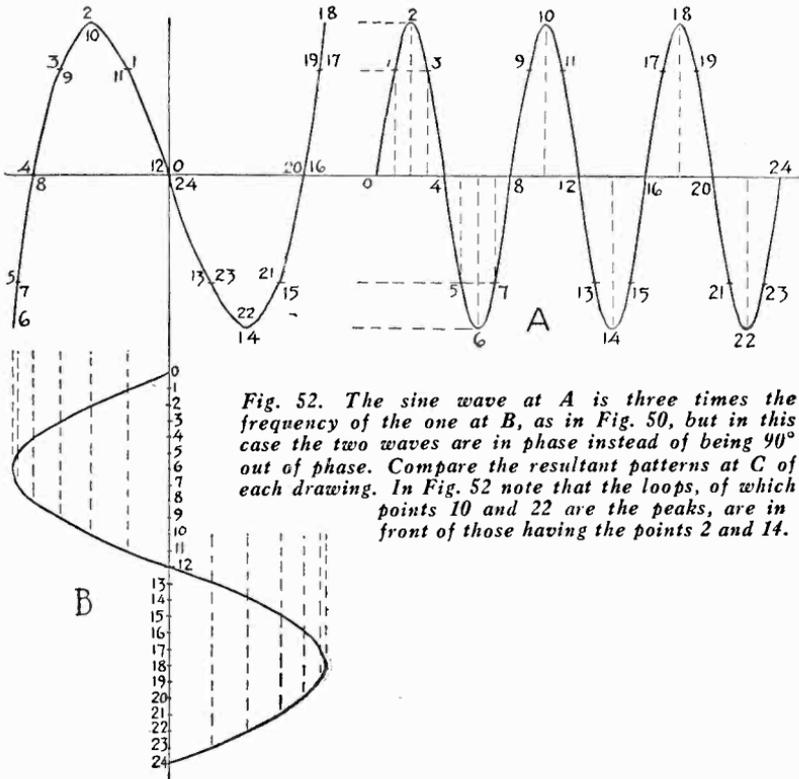
Fig. 52. The sine wave at A is three times the frequency of the one at B, as in Fig. 50, but in this case the two waves are in phase instead of being 90° out of phase. Compare the resultant patterns at C of each drawing. In Fig. 52 note that the loops, of which points 10 and 22 are the peaks, are in front of those having the points 2 and 14.
