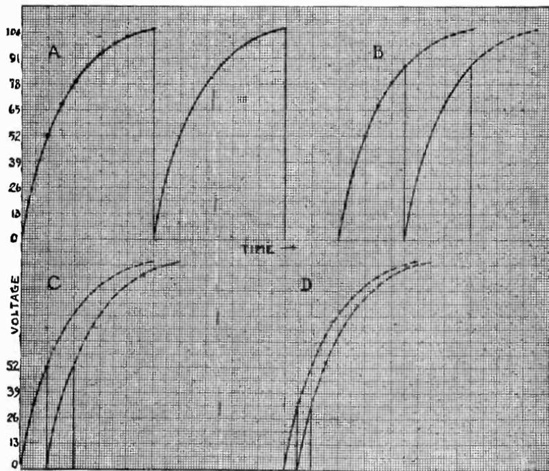
*Fig. 33-A. Two cycles of a theoretical saw-tooth wave such as would be developed by a resistor-condenser-discharge tube combination with the tube tripping at 105 volts. Fig. 33-B shows the waveform when the tube flashes at 37.7 volts and Fig. 33-C shows the wave when the tube flashes at 52 volts. When the flashing voltage is reduced to 32.5 volts, Fig. 33-D, the charging portion of the wave is fairly linear.*
