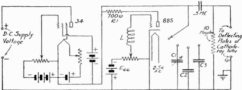
*Fig. 38. The type 34 tube replaces the resistor,  $R$ , (Fig. 34) as a current limiting device in this relaxation oscillator sweep circuit. The constant current flow tends to charge whatever condenser is in the circuit at a constant rate, making the voltage rise constant thereby supplying a linear output to the deflecting plates.*
