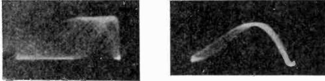
*Fig. 71, left, Fig. 72, right. The pattern shown in Fig. 72 resulted from adjusting the synchronization control a trifle after the pattern in Fig. 71 was photographed. The pattern in Fig. 72 is still under-synchronized.*
