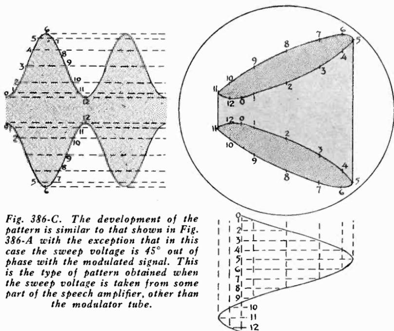
*Fig. 386-C. The development of the pattern is similar to that shown in Fig. 386-A with the exception that in this case the sweep voltage is  $45^\circ$  out of phase with the modulated signal. This is the type of pattern obtained when the sweep voltage is taken from some part of the speech amplifier, other than the modulator tube.*
