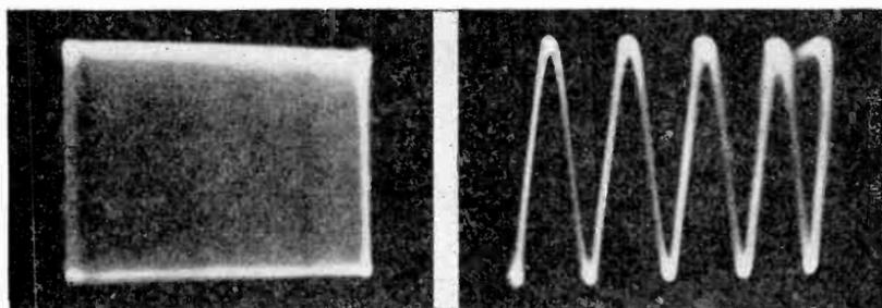
*Fig. 243, left, Fig. 244, right. After corrective measures were taken with the oscillator used to generate the patterns shown in Figs. 241 and 242, the pattern of Fig. 243 indicated that distortion had been removed from the carrier, because the streaks had disappeared. The oscillogram of Fig. 244 shows the corresponding carrier wave, which has little of the distortion of Fig. 242.*
