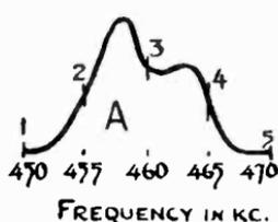
*Fig. 263. Development of an asymmetrical resonance curve of an i-f. transformer. The sweep circuit is so synchronized with the output of the frequency modulated oscillator that the lowest frequency, 450 kc., is at the start of the sweep and the highest frequency, 470 kc., occurs at the middle of the sweep.*
