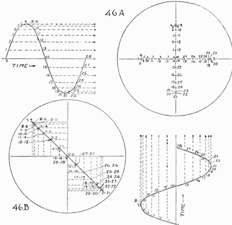
Fig. 46. The sine wave at the left is impressed on the vertical plates and the one below is impressed on the horizontal deflection plates. Each spot on the screen bears two numbers, except the peaks, as the voltage varies from zero to maximum and returns. The resulting figure is shown in Fig. 46-B. These waves are in phase.
