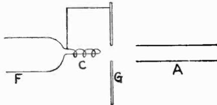
the current flowing through the cathode is varied by means of a rheostat and thereby controls the emission. The shield or electron gate G is electrically connected to the cathode at one point. The anode A is connected to a fixed voltage source, which applies a positive voltage to this electrode. Further, a certain amount of inert gas is placed within the glass envelope.
