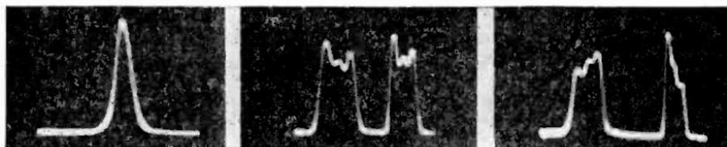
*Figs. 268, left, 269, middle, 270, right. The sweep frequency used in developing the symmetrical pattern of Fig. 268 was twice the motor frequency. Compare with Fig. 265. Figs. 269 and 270 are examples of asymmetrical resonance curves. Explanation of the dissimilarity of the curves is given in the accompanying text.*
