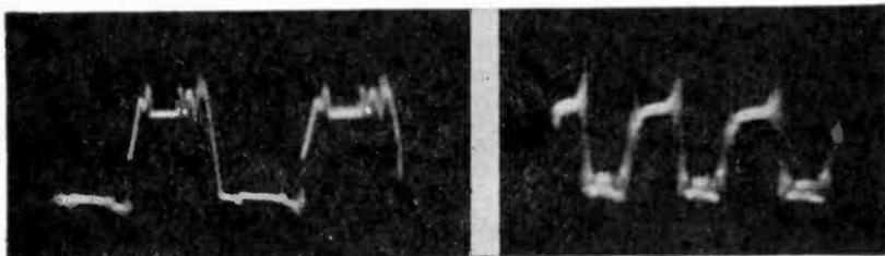
*Figs. 374, left, 375, right. The effect of maximum and minimum separation between the secondary contacts is shown in Figs. 374 and 375 respectively.*
