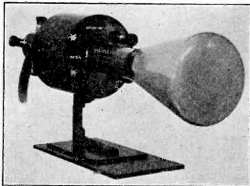
*Fig. 24D. Magnetic deflection apparatus. The circular housing contains the four coils, which are brought close to the tube's neck when it is inserted in the opening. The lead at the rear connects the tube's base to its socket in the oscillograph so that its power supply unit can be used.*
