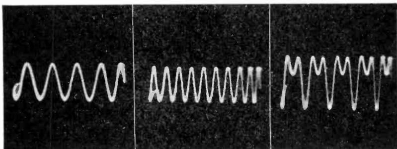
*Figs. 154, left, 155, middle, 156, right. A 1000-cycle sine wave, shown in Fig. 154, and a 2000-cycle sine wave, Fig. 155, result in the composite wave, Fig. 156. Note that the 2000-cycle wave (the second harmonic of the 1000-cycle wave) is almost equal in amplitude to the fundamental frequency. Compare the amount of the dip in Fig. 156 with that of Fig. 157.*
