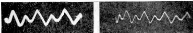
*Figs. 372, left, 373, right. Oscillogram of voltage taken across V and V<sub>1</sub> is shown in Fig. 372. Fig. 373 shows the voltage across the same points, but with a shorter exposure of the photographic film. Note the transients in Fig. 372, indicated by the faint vertical lines below the wave, but not visible in Fig. 373.*
