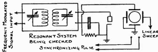
*Fig. 280. Arrangement of apparatus for obtaining alignment curves. Rectification occurs in the diode and the voltage across the diode load is impressed on the vertical plates of the tube. This voltage depends on the signal voltage built up across the resonant circuit.*
