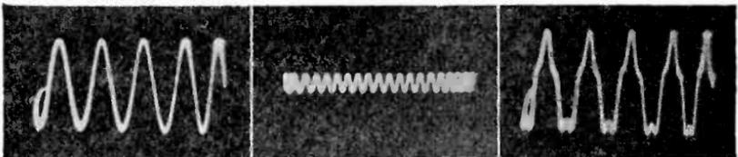
*Figs. 170, left, 171, middle, 172, right. The 1000-cycle wave, Fig. 170, is the fundamental and the 4000-cycle wave, Fig. 171, is its fourth harmonic. The composite wave is shown in Fig. 172. Compare with Fig. 167 for changes in the shape due to the substitution of the fourth for the third harmonic.*
