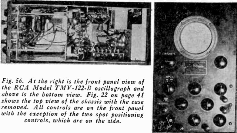
*Fig. 56. At the right is the front panel view of the RCA Model TMV-122-B oscillograph and above is the bottom view. Fig. 22 on page 41 shows the top view of the chassis with the case removed. All controls are on the front panel with the exception of the two spot positioning controls, which are on the side.*
