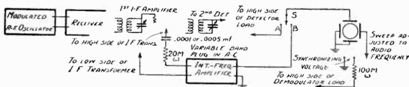
Fig. 195. Circuit for checking overloading in i-f. amplifiers.
