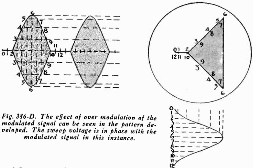
*Fig. 386-D. The effect of over modulation of the modulated signal can be seen in the pattern developed. The sweep voltage is in phase with the modulated signal in this instance.*
