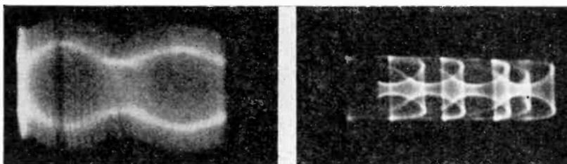
Fig. 431 (left) is an example of hum modulation of the carrier, which is modulated at 1000 cycles. Fig. 432 (right) is an example of a pattern resulting from incorrect test connections.
