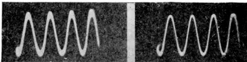
*Figs. 199-A, left, 199-B, right. The broadness of the waveshapes in Fig. 199-A indicates that some r-f. is present in the output of the demodulator. The oscillogram in Fig. 199-B was made after filtering out the r-f. Note the difference in the peaks.*
