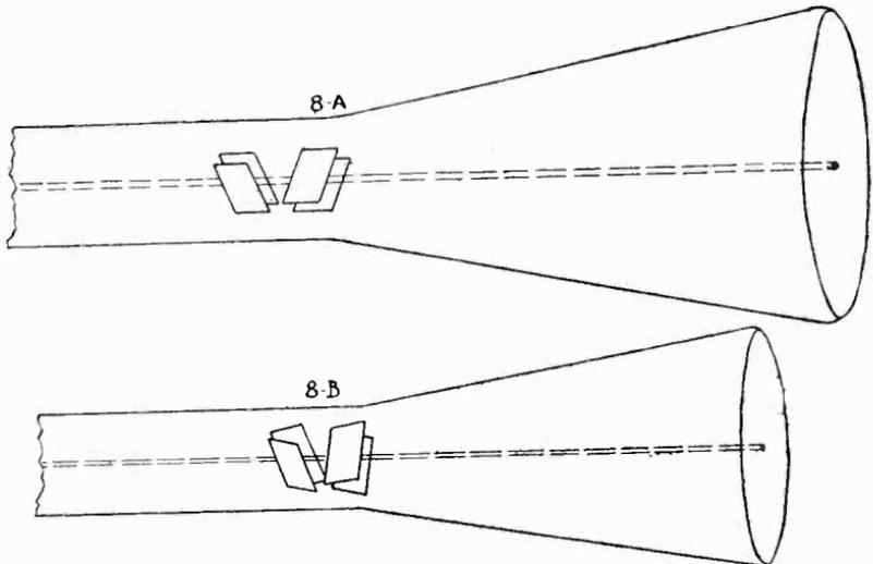
*Fig. 8A shows the relative position of the deflecting plates of a Western Electric type of cathode-ray tube. Note that each pair of plates is parallel. Fig. 8B shows how the plates of an RCA tube are at an angle to each other. It should be noted that the longer sides of each pair are perpendicular in both tubes.*
