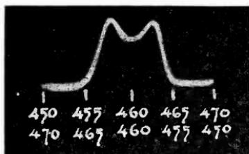
*Fig. 273. The circuit used for obtaining the oscillogram of Fig. 272 was adjusted so that it was symmetrical and the resonance curve then taken. The result is shown at the left. Note that now the two curves coincide throughout.*
