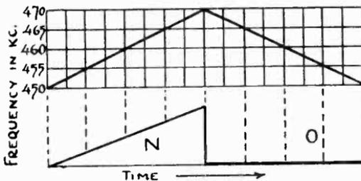
*Fig. 275. During one half of each revolution of the variable condenser in the frequency modulator of Fig. 256, the sweep circuit is shorted and only cycle N spreads the resonance curve, giving a single instead of a double pattern.*
