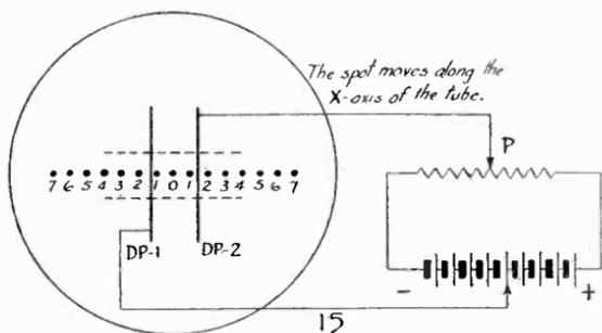
*Fig. 15. The horizontal positioning of the spot is accomplished in the same way as it was moved vertically in Fig. 14. Note that in this and other figures the seven spots indicate ANY positions of the beam's trace in the directions indicated.*
