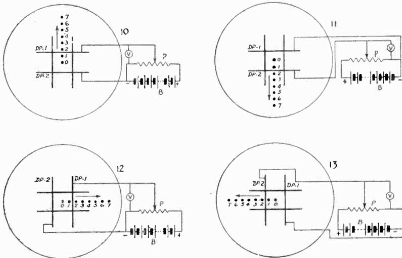
*Figs. 10, 11, 12, 13. The circles indicate the viewing screen of a cathode-ray tube. The dots, numbered 0 to 7, show the successive positions of the spot formed by the electron beam when it strikes the screen and various voltages are applied to the deflecting plates, the voltages from the battery, B, being controlled by a potentiometer, P, and their values being read by the voltmeter, V.*
