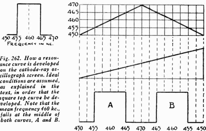
Fig. 262. How a resonance curve is developed on the cathode-ray oscillograph screen. Ideal conditions are assumed, as explained in the text, in order that the square top curve be developed. Note that the mean frequency 460 kc., falls at the middle of both curves, A and B.
