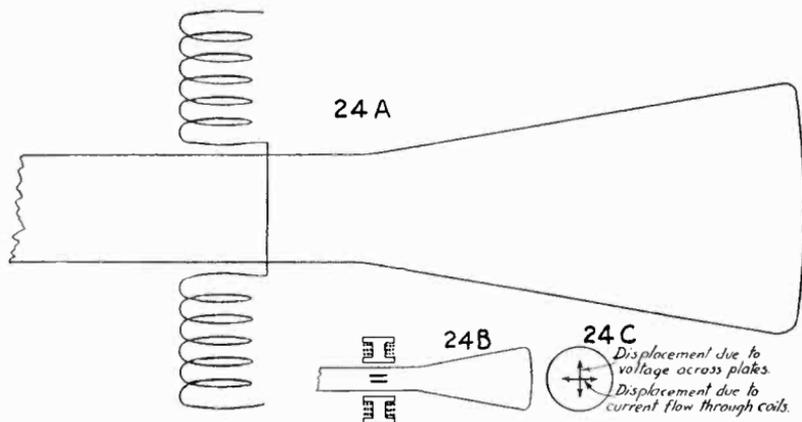
*The two coils connected in series (Fig. 24A) are shown in their positions relative to the plates of the tube (Fig. 24B). The displacement of the beam due to voltage across plates is perpendicular to the displacement due to current flow through the coils. (Fig. 24C.)*
