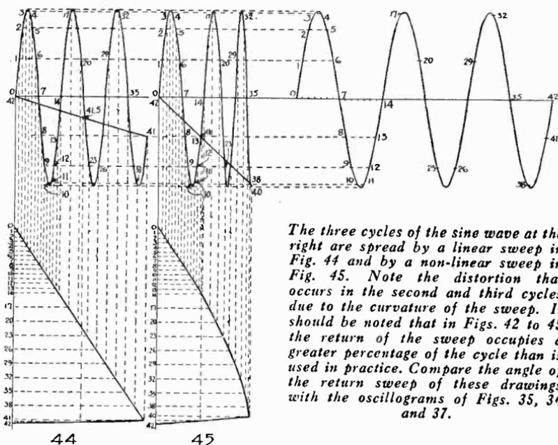
*The three cycles of the sine wave at the right are spread by a linear sweep in Fig. 44 and by a non-linear sweep in Fig. 45. Note the distortion that occurs in the second and third cycles due to the curvature of the sweep. It should be noted that in Figs. 42 to 45 the return of the sweep occupies a greater percentage of the cycle than is used in practice. Compare the angle of the return sweep of these drawings with the oscillograms of Figs. 35, 36 and 37.*
