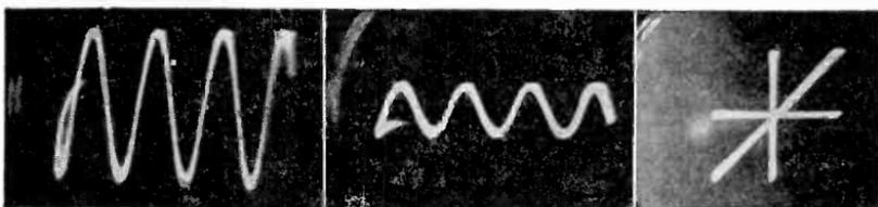
*Figs. 207, left, 208, middle, 209, right. The output wave of the Class A stage is shown in Fig. 207. The input voltage wave to the Class B stage is shown in Fig. 208. The correct phase relation of 180° between the two voltages to the Class B input is indicated in Fig. 209.*
