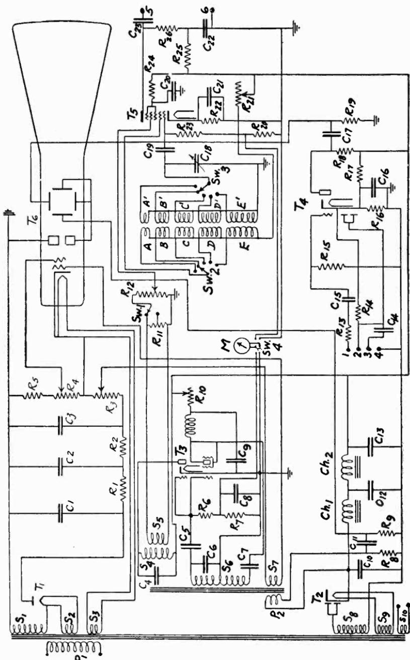
Fig. 279. Schematic diagram of the Egert Model VRO oscillograph.
