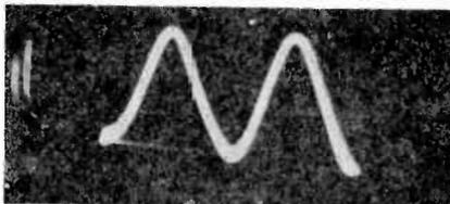
An increase in the sweep frequency, in order to show two waveforms upon the screen, produced the pattern shown in figure 136. (The vertical deflection, that is, the voltage being observed, was applied
