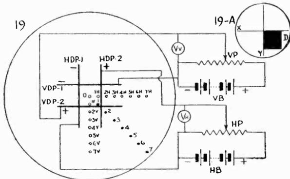
*Fig. 19. The positions of the beam's spot are within quadrant D, when plates VDP-2 and HDP-2 are made positive with respect to VDP-1 and HDP-1 respectively. See Fig. 19-A for the portion of the screen covered.*
