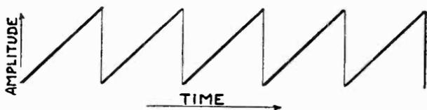
*Fig. 32. The ideal saw tooth wave. Note that the charging portion of each cycle of this wave is linear, i.e. a straight line, indicating a constant increase in voltage with respect to time. The discharge from maximum to zero voltage is perpendicular, indicating an instantaneous return to the starting point.*
