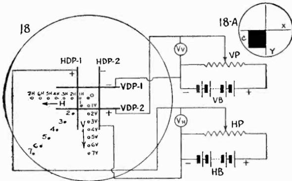
*Fig. 18. To position the spot anywhere within quadrant C, the plates VDP-2 and HDP-1 are made positive with respect to their respective plates. See Fig. 18-A for the area covered in this particular case.*
