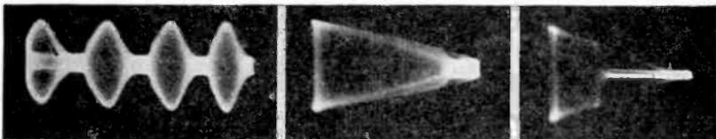
*Fig. 413 (left) indicates the modulated wave during excessive regeneration and Fig. 414 (middle) shows the equivalent trapezoidal pattern. Fig. 414-A (right) is another trapezoidal pattern indicating improper neutralization adjustment.*
