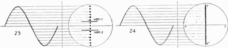
*Fig. 23. The change in polarity of an a-c. voltage sine wave, when connected to the vertical deflection plates, will cause the spot to assume the positions indicated by the series of vertical dots. No voltage is impressed on the horizontal deflecting plates.*
