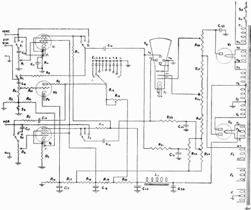
*Schematic diagram of the Triumph Model 800 cathode-ray oscilloscope. Note the two rectifiers, the type 879 supplying the high voltages for the cathode-ray tube, type 906, and the type 80 supplying the bias and plate voltages for the remainder of the tubes.*
