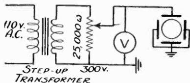
*Fig. 150. Schematic diagram of the circuit used for determining the voltage sensitivity of a cathode-ray tube. This is found by measuring the length of the line on the screen, noting the voltage on V and following the directions given in the text.*
