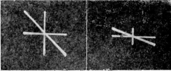
*Fig. 93-C, left, Fig. 93-D, right. A phase difference of  $0^\circ$  exists between the two voltages. In C equal amplitudes on both axes give the pattern a  $45^\circ$  angle with the horizontal, but when the horizontal*
