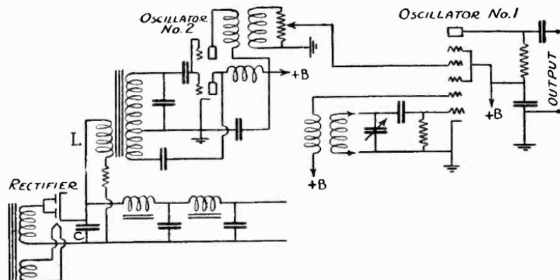
Fig. 253. Schematic diagram of a frequency modulated oscillator, wherein the spreading of the frequency over a band is accomplished by using the variation in permeability of the iron core in the No. 2 oscillator oscillation transformer.
