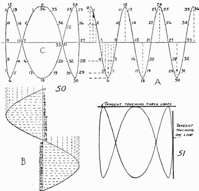
Fig. 50. The sine wave at A is three times the frequency of that at B and is  $90^\circ$  out of phase. Both waves are divided into equal time intervals. The numbers on the resultant image at C indicate the amplitude displacement of each wave at the same instant.
