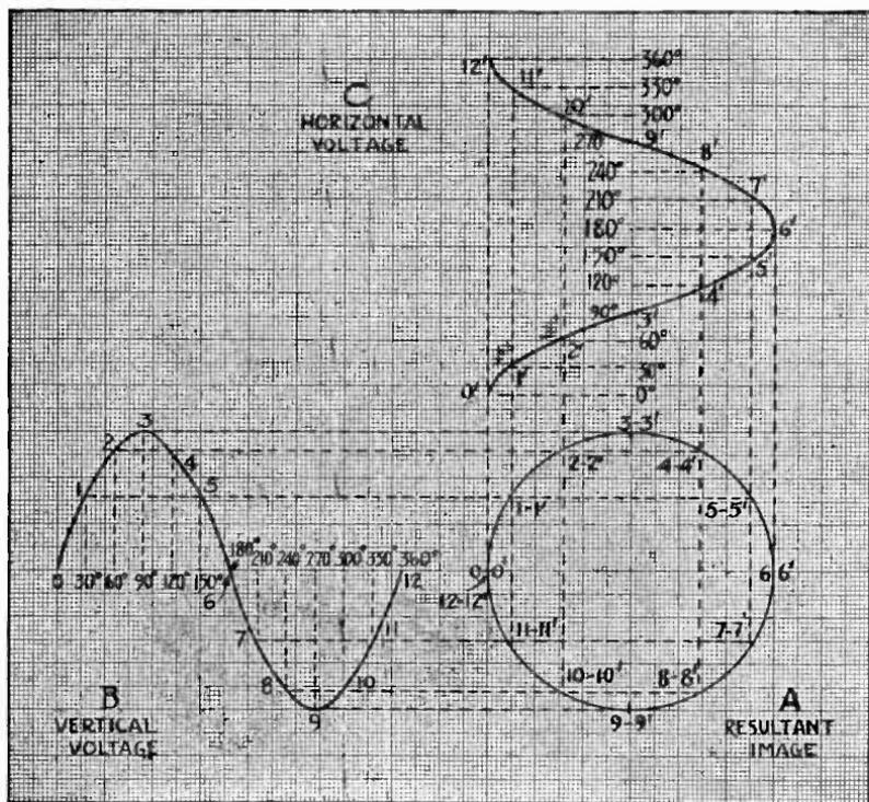
Fig. 48. The sine wave at B is  $90^\circ$  out of phase with the one shown at C, so that the resulting pattern is a circle. Note that the time axis here is divided into degrees of a circle instead of fractions of a second as in previous drawings.
