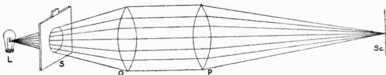
*Fig. 5. A sketch of an optical system that is analogous to the elements of an RCA cathode-ray tube. L is a light source, whose output can be controlled by the variable opening of the shutter S. O and P are lenses, which concentrate the beam to a spot on the screen Sc.*
