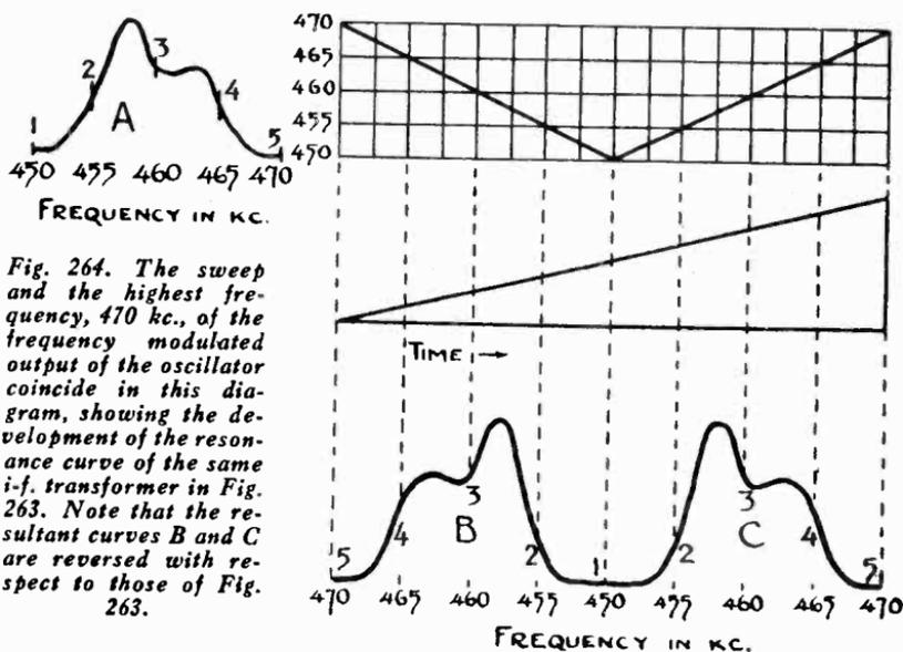
Fig. 264. The sweep and the highest frequency, 470 kc., of the frequency modulated output of the oscillator coincide in this diagram, showing the development of the resonance curve of the same i-f. transformer in Fig. 263. Note that the resultant curves B and C are reversed with respect to those of Fig. 263.
