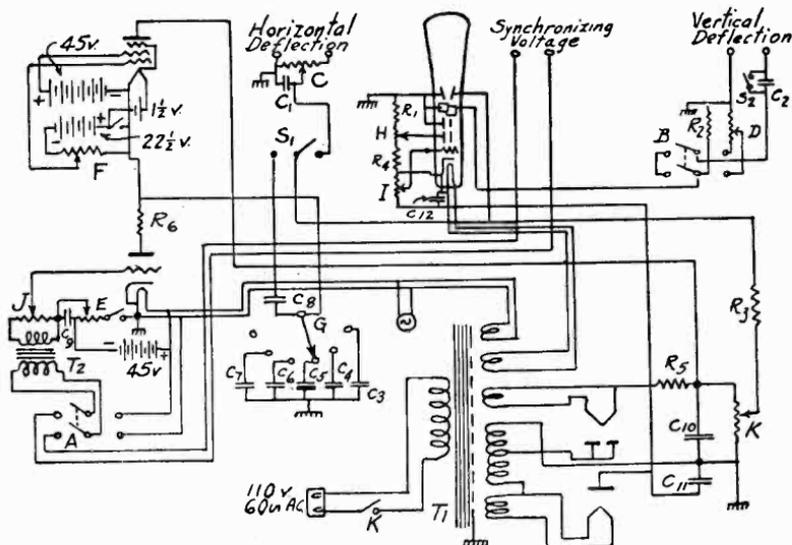
Fig. 59. The schematic diagram of the Kaltman-Romander oscillograph.
