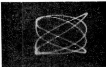
Figures 101-A and 101-B illustrate 5-1 ratios, but it would be most difficult to anyone but an experienced person to determine that figure 101-B indicates a 5-1 ratio, because the loops have been covered by other loops. On the other hand, the pattern of 101-A shows all of the
