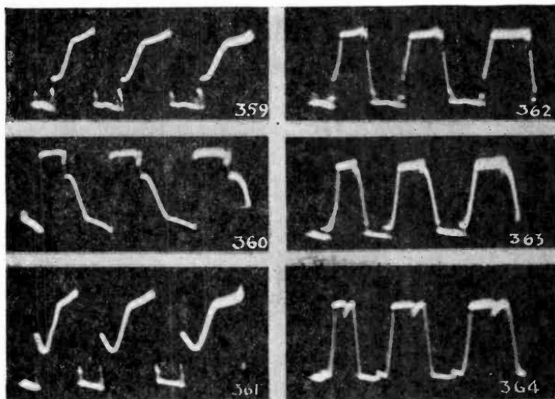
*Figs. 359 to 364. Oscillograms in Figs. 359, 360 and 361 were made with the vibrator of Fig. 353 functioning as a half-wave rectifier by disconnecting contact A. Oscillogram made when contact A was restored to normal operation is shown in Fig. 362. When both contacts were opened to maximum separation, oscillograms in Figs. 363 and 364 were obtained across P1 and S1 and their respective center taps.*
