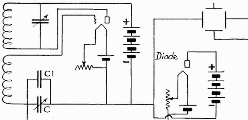
*Fig. 40. This circuit is capable of producing frequencies of a fairly high order. It is an ordinary oscillator circuit so arranged that the grid circuit will block periodically. The filament temperature of the diode is the rough frequency adjustment and the condenser C is the fine frequency adjustment.*
