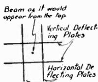
*Fig. 3. If it were possible to see through the screen at the tube's end, the electron stream would appear as a small dot in the middle of a square formed by the two sets of deflection plates, on which no deflecting voltage was impressed.*
