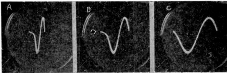
*Fig. 67. The sine-wave voltage impressed on the vertical plates and the sweep voltage are both 700 cycles, resulting in the appearance of a single cycle on the screen. In A and B, the sweep amplitude is insufficient to give a true image; whereas in C the wave is spread out enough to present a substantially undistorted image.*
