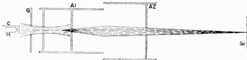
*Fig. 6. The path of the electron stream through an RCA cathode-ray tube is here shown. The heater, *H*, warms the cathode, *C*, from which the electrons are emitted. The stream is concentrated and accelerated by the two anodes, *A1* and *A2*, finally appearing as a spot on the screen, *Sc*. See Fig. 5 for optical analogy.*
