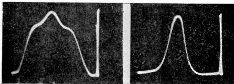
*Fig. 276, left, Fig. 277 right. The resonance curve in Fig. 276 is non-symmetrical and that in Fig. 277 is symmetrical. These oscillograms were made using the frequency modulator and sweep described in Fig. 275. The vertical line on the right of each oscillogram indicates the vertical displacement due to change in frequency, but as the sweep was shorted, it is not spread across the screen.*
