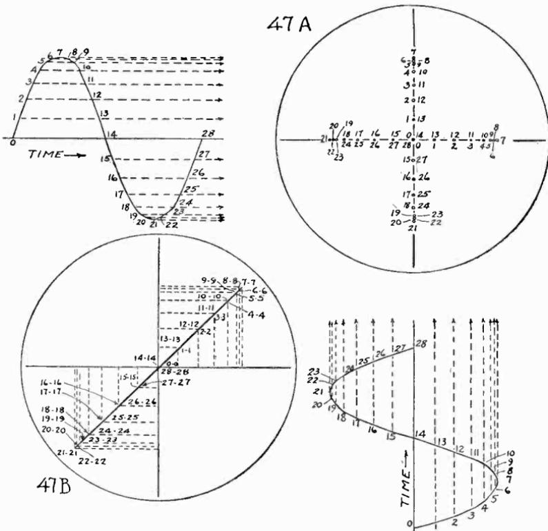
Fig. 47. The development of the resulting image seen on the screen in Fig. 47-B is the same as Fig. 46, but in this case the two sine waves impressed on the deflecting plates of the tube are 180° out of phase; hence the image slopes to the right instead of the left, as in Fig. 46.
