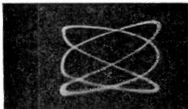
Figure 100 shows a 4-3 ratio pattern. Note the four loops on one side and the three loops on the other side. At the same time, we want to call to your attention the fact that often the loops are more distinct upon one side of the pattern than upon the other. For example, the
