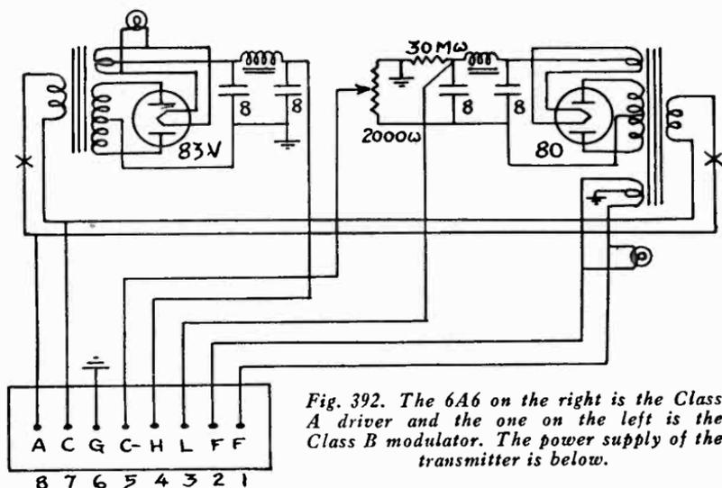
Fig. 392. The 6A6 on the right is the Class A driver and the one on the left is the Class B modulator. The power supply of the transmitter is below.
