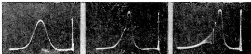
*Figs. 320, left, 321, middle, 322, right. A correct resonance curve for a single-peaked system with minimum regeneration is shown in Fig. 320. An increase in regeneration caused the curve to become asymmetrical, see Fig. 321. Actual generation of oscillations is indicated in Fig. 322.*
