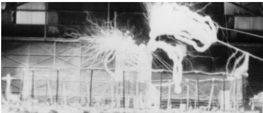
“Magnifying transmitter” constructed by Robert Golka, following the specifications of Tesla’s 1899 apparatus at Colorado Springs. See Fig. 1b for circuit diagram. Energized, as shown, it produced electrical discharges estimated at 12.5 million volts. Note that the extra coil is located at the centre of the excitation transformer. (Photo courtesy Tesla Wardenclyffe Project).
