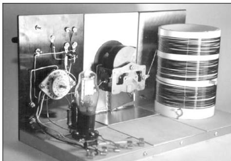
Fig. 4. Here's the interpanel set I hinted at in my first column. It's grown to three panels and I'll soon be adding a Fleming valve detector.
