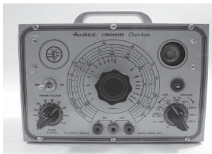
Fig. 29. C-1 Condenser Checker, Type 1. Toggle on-off switch.
