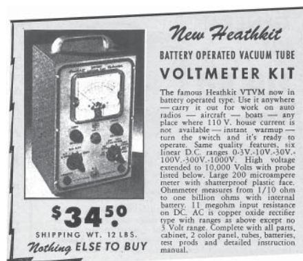
Fig. 16. V-3 Battery Powered VTVM (Radio News, March 1949, pg. 73)
