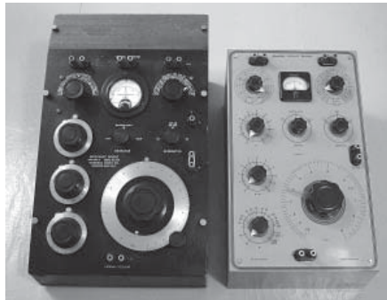
Fig. 26. IB-1 with General Radio 630-A. The IB-1 has 10-0 main dial and C-R-L below the main dial and multiplier switch.
