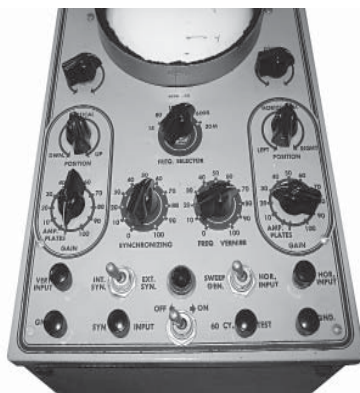
Fig. 11. O-3 Oscilloscope, Type 1 Aluminum handle. Note "AMP. PLATES" on both gain controls.
