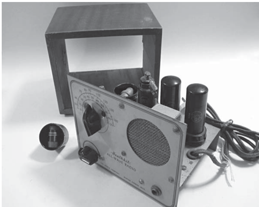
Fig. 22. K-2 All Wave. Note case, broadcast and short wave coils, war surplus tubes.
