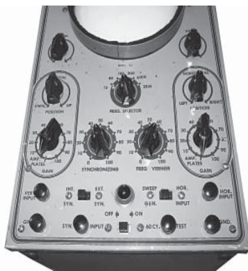
Fig. 12. O-3 Oscilloscope, Type 2 Slide switches
