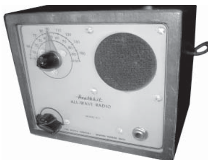
Fig. 24. Probable Last Version of K-2 with vernier tuning. Jay Whipple, Jr. collection.
