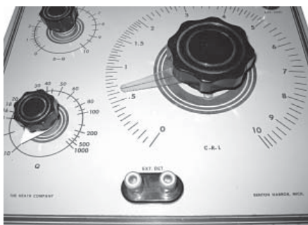
Fig. 28. IB-1B 0-10 main dial and C-R-L below main dial and multiplier switch.
