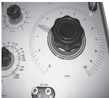
Fig. 27. IB-1A 0-10 main dial and L-R-C below main dial and the multiplier switch.
