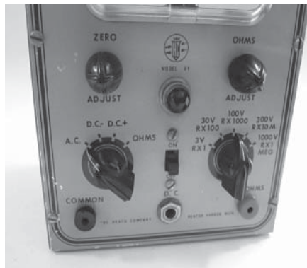
of circuits under test. The meter is a 500 microampere movement, and the circuit uses 1% precision resistors. The ohmmeter measures one tenth of an ohm to one billion ohms. It came in three types, only two of which were advertised. The Type 1 has the khaki painted brass handle, a toggle on-off switch and 5 ranges. It was advertised December 1947 through June 1948 (Fig. 13). The Type 2 had a polished aluminum handle and a longer bat-handle toggle switch on most. The Type 2 was advertised for nine months, starting in July 1948. The Type 3 was like the Type 2 except it has a slide on-off switch (Fig. 14). I believe it was produced at the end of the V-1 production run, probably in March 1949. It was never advertised but is in my
