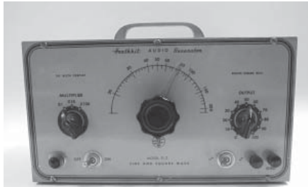
Fig. 18. G-2 Sine and Square Wave Audio Generator, Type 2, Toggle Switch
