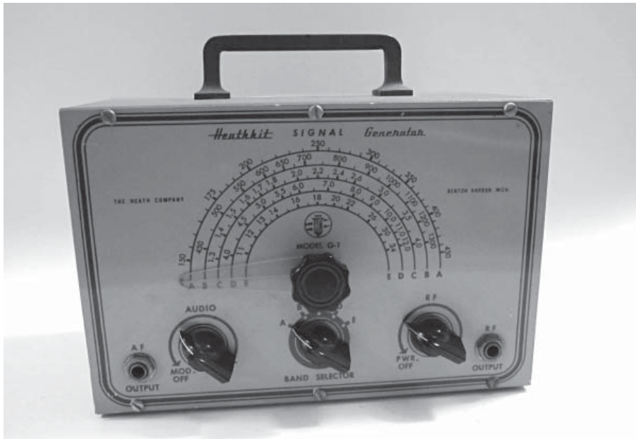
Fig. 17. G-1 Signal Generator, Type 1. Has Earliest Handle.
