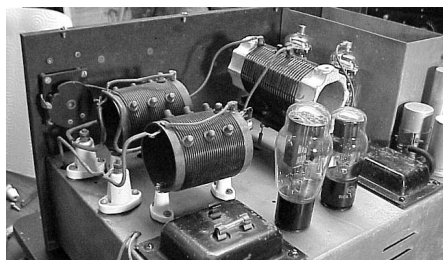
Interior view showing repaired antenna coils.
