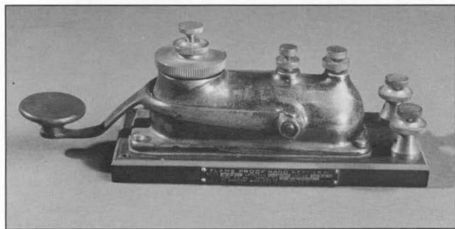
Figure 91. Type SE-86 flame proof 1/2-kW hand key. This well built spark key is rated at 5 amperes and was designed for use where open spark is not permitted, i.e., an airplane cockpit.
