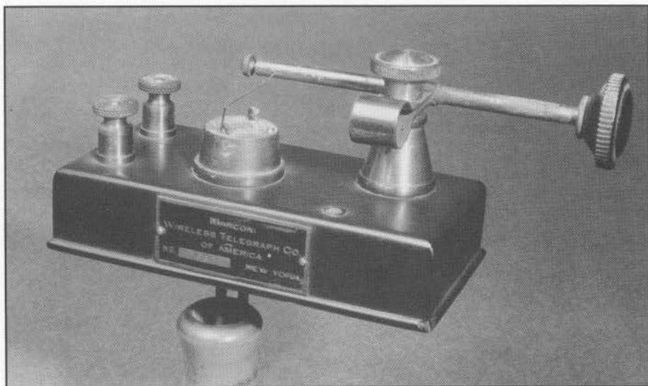
Figure 82. The external crystal detector for the Type 103 receiver. It uses a cup containing both carborundum and cerusite minerals. A brass loop is incorporated, which, when locked onto an operating table, made it difficult to put in your pocket for your own use. Source: Kreuzer Collection
