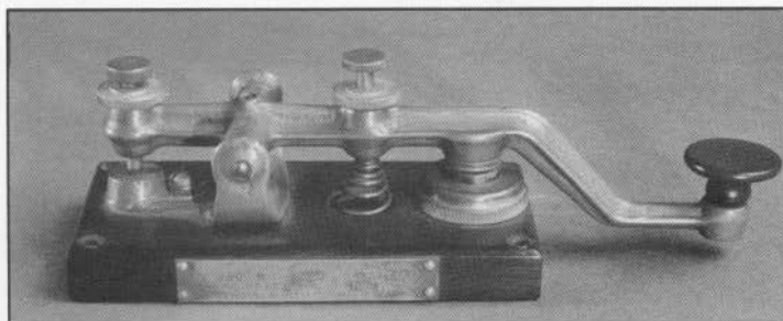
Figure 100. Type SE 68 auxiliary hand key, made for the U.S. Navy. Produced in 1917, this key is rated at 20 amperes @ 250 volts.
