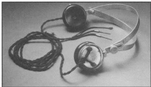
Figure 105. A pair of American Marconi headphones, identified on the earpiece. Note the Navy type headband and the length of the phone pins. This set may have been used at the Aldene factory.
