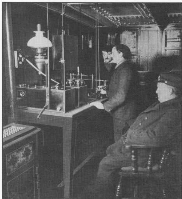
Figure 17. An early ship-board wireless station aboard the lightship Tongue in 1900. It used the Marconi coherer receiver and the 10" spark coil.
