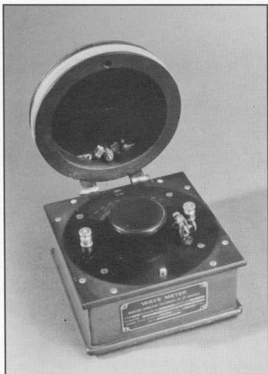
Figure 84. Marconi Type 22 wavemeter, covering from 200 to 750 meters. It is dated 5/20/14 on the nameplate.
