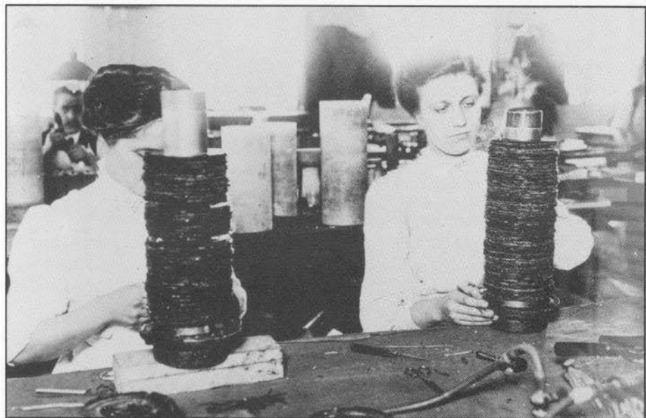
Figure 31. Women assembling various sections of the 10" induction coil at the Chelmsford Works. The forms for pouring the insulating wax can be seen in the background.
