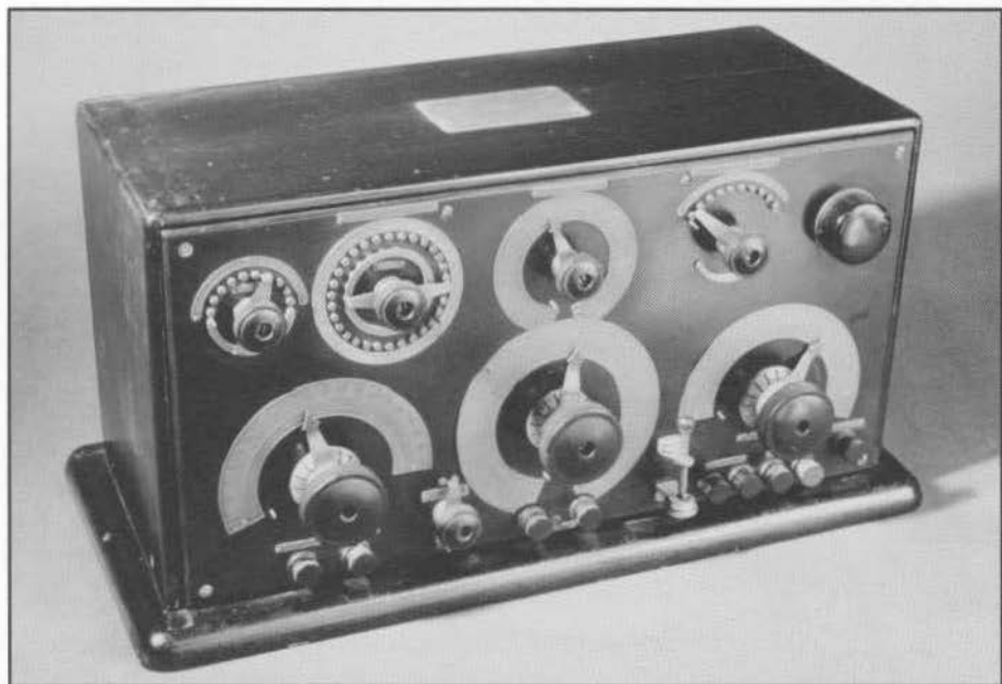
Figure 87. Marconi Type 106 receiver, probably the most popular of all Marconi receiving sets. It lasted for many years, going through numerous changes in both design and type numbers (106B, 106C, 106D).
