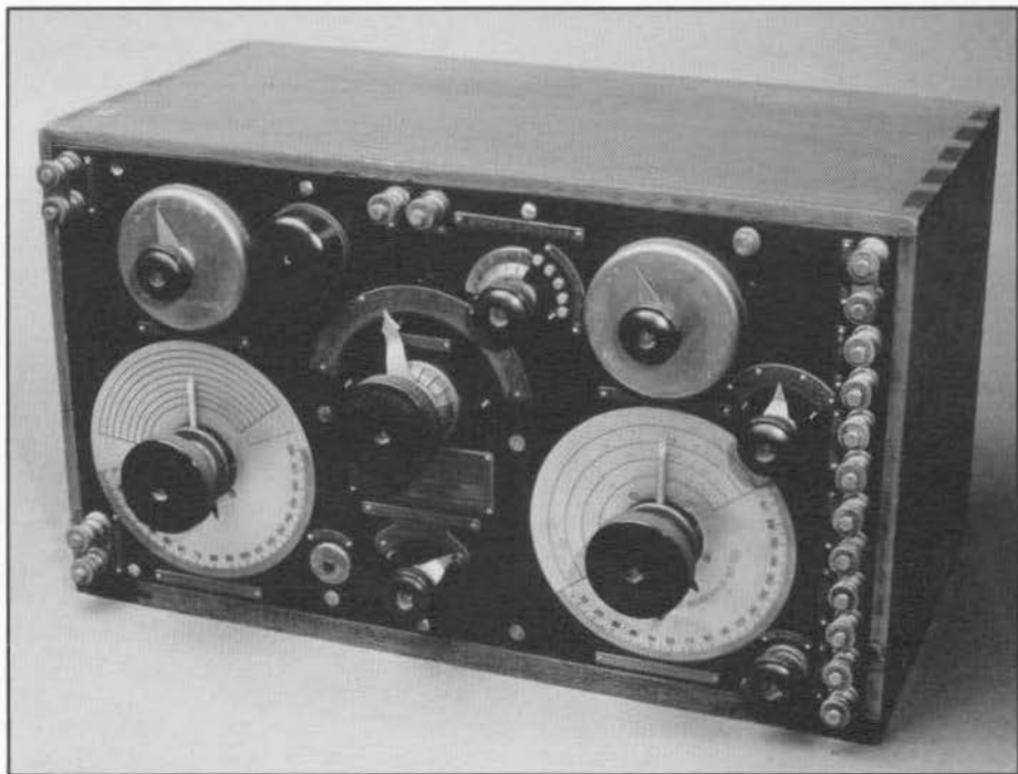
Figure 96. Marconi Type CM 2946C Short Wave receiver made for the Navy Department, Bureau of Steam Engineering. It covered from 250 to 3100 meters and was built in 1917. A popular battleship receiver, many were manufactured during the First World War.
