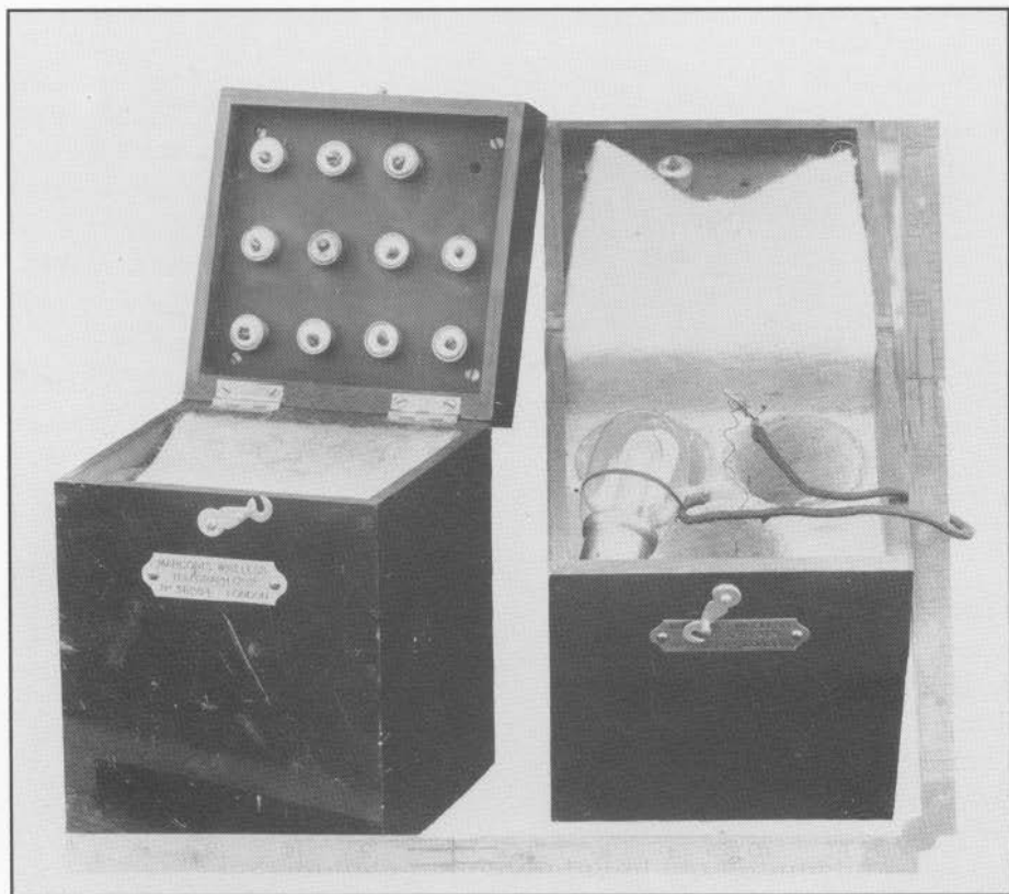
Figure 54. A spare parts kit that includes various types of crystals as well as extra Fleming Valves. These boxes would have accompanied the tuner in Figure 53. Source: Kreuzer Collection
