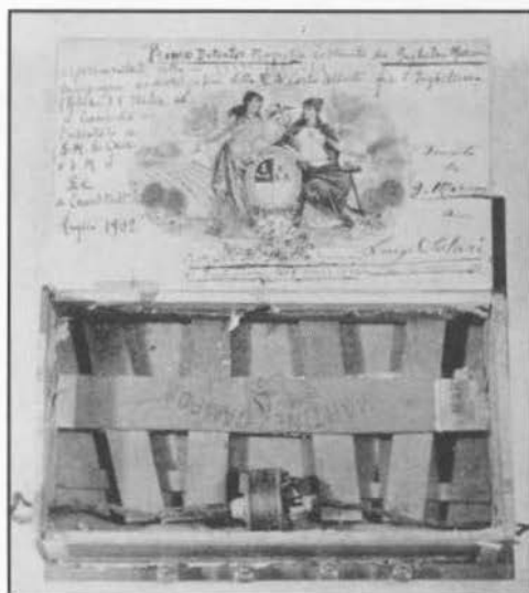
Figure 38. A prototype of Marconi's magnetic detector, used aboard the Italian Navy ship Carol Alberto in 1902. It was constructed in an ordinary cigar box. Source: Luigi Solari, Marconi, 1940
