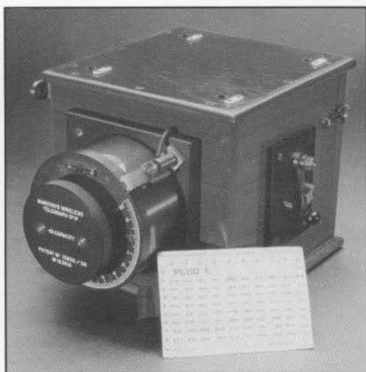
Figure 65. Early form of wavemeter incorporating an internal battery and wave-length chart, circa 1909.
