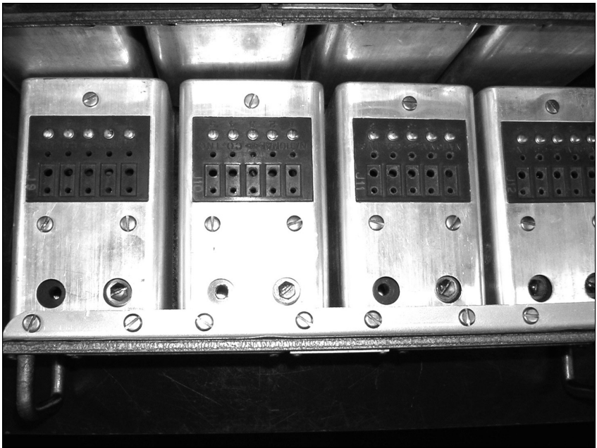
Figure 21. This close-up of the RBJ 00 coil insulators shows how a typical HRO coil module was constructed. (Author's collection.)
