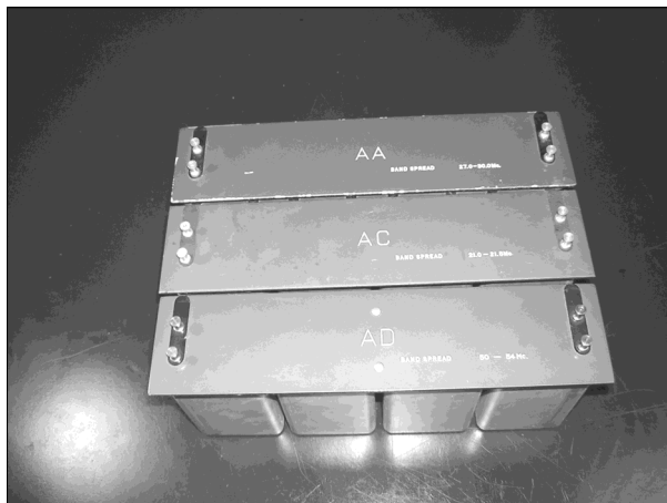
Figure 29. Coils for the HRO-50. These coils are sleeker looking than those for earlier HROs. (Author's collection.)
