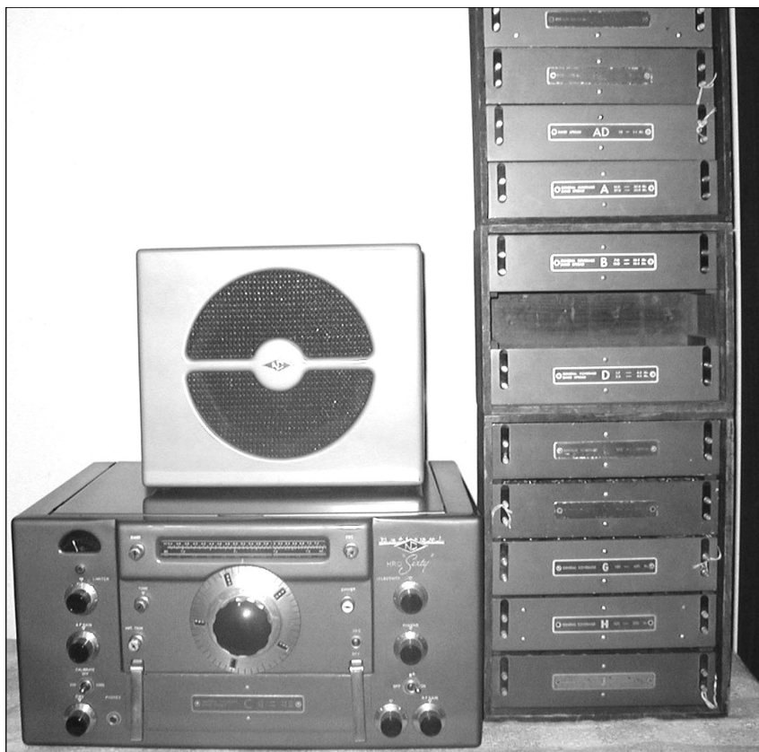
Figure 31. The HRO-60, introduced in 1952, was the last of the vacuum tube HROs. A full set of coils for an HRO takes up a lot of space, as this photo shows. (Author's collection.)
