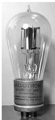
Left: Early transmitting tube— RCA UV-202, 5 watt.
