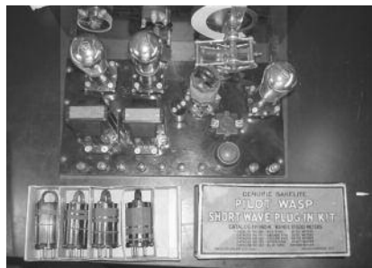
Wasp interior with coilset. One coil is installed in radio.
