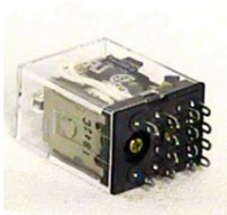
Main Chassis Relays RL1 & RL2 FRL263-DO12/04CS or Guardian Type 1315H (4PDT 5 AMP Contacts) Size: just over 1 cubic inch
