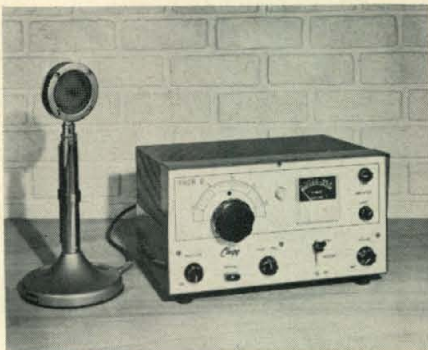
View of the receiver and r.f. unit. Controls are (left to right) BFO INJECTION, crystal socket, receiver-v.f.o. tuning dial (above), VFO-XTAL switch, SEND-RECEIVE-ANL, and (top to bottom, far right) final plate tuning, antenna loading and ON-OFF-VOLUME. The Thor 6 50 mc transceiver runs 60 watts input and is v.f.o. controlled. Not shown in photo is the modulator and power supply unit, located remote and connected by a 10 foot cable.
