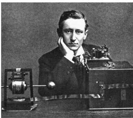
Publicity photo of Guglielmo Marconi posing with his early radio apparatus. Spark transmitter is on left, coherer receiver on right.
