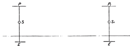
Fig. 29. Tesla morphed the description of his 1893 experimental configuration shown in Fig. 27 by claiming in 1900 that S_1 in circuit ES_1P_1 to the right of this figure represents a receiver, not a second source. ( Century Magazine , Vol. 60, June 1900, p. 206)
