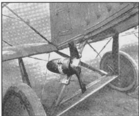
Figure 30. Wind-driven generator to power radio equipment, fitted to a Curtiss J.N. "Jenny" trainer.
