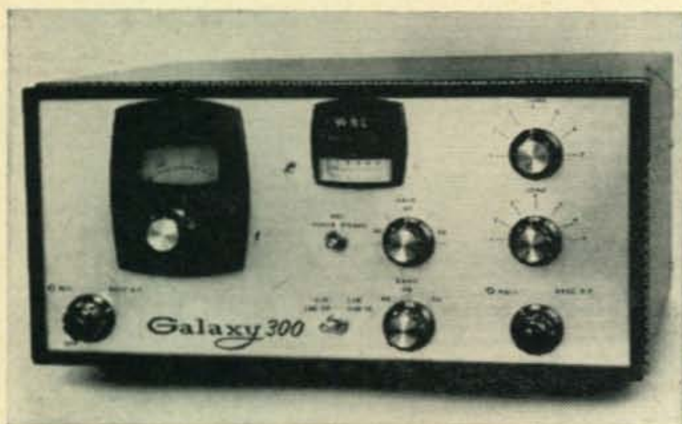
The Galaxy 300 s.s.b. transceiver for operation on the 20, 40 and 80 meter phone bands with selection of either upper or lower sideband at 300 watts p.e.p. input.
