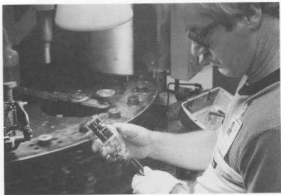
Fig. 11. Adding the base.
