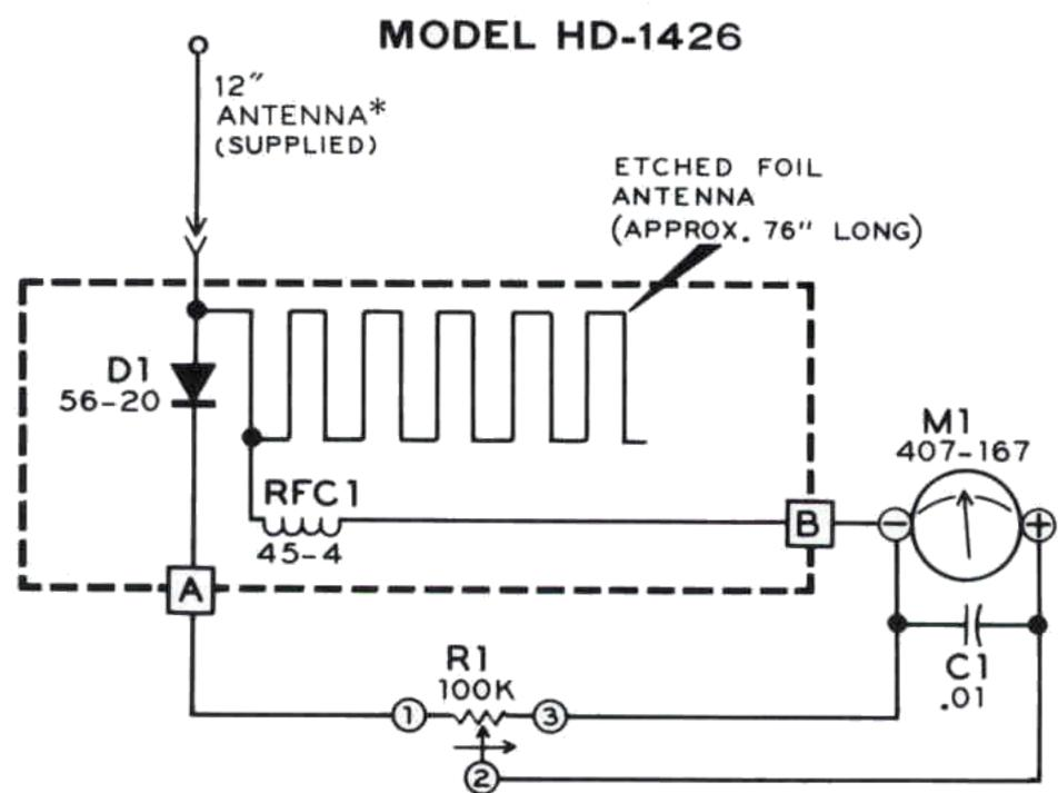
\*NOTE: YOU may use any desirable added wire for increased instrument sensitivity.
