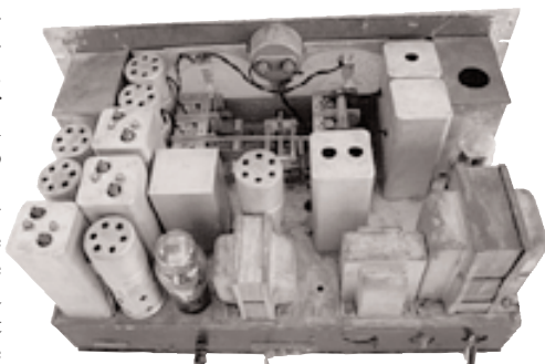
Top view of the receiver. Note the high density of the layout. There is very little room for any additions above the chassis.
