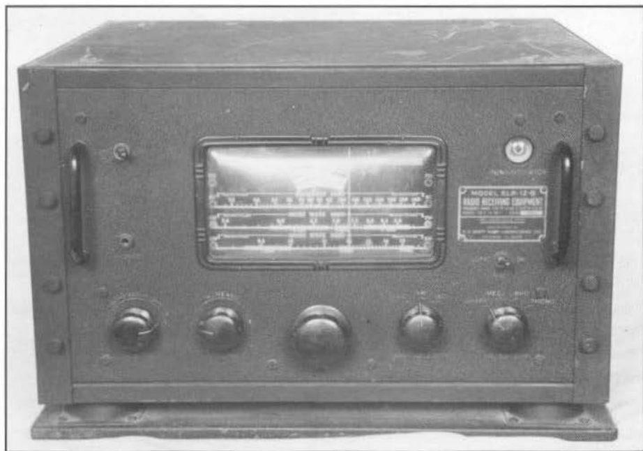
Figure 71. SLR-12B. Although most Merchant Marine sets had a Navy variant, the SLR-12B is an exception
