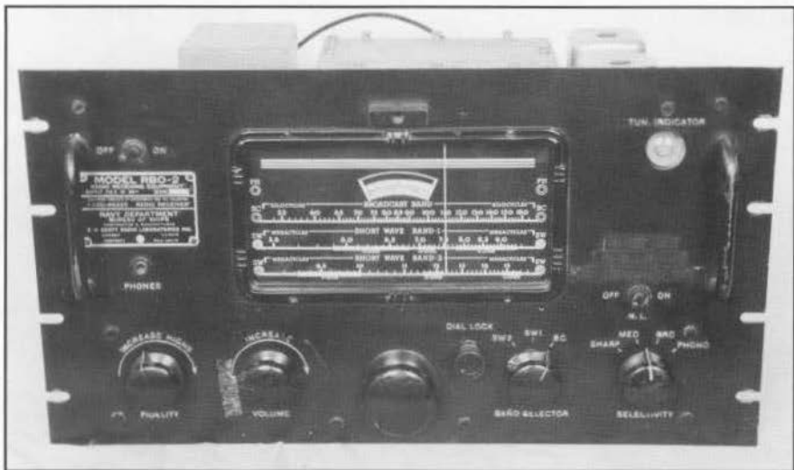
Figure 68. RBO-2. The RBO family had several variations, differing only slightly in tube lineups.
