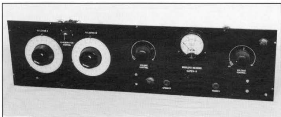
Figure 2. Front view of World's Record Super 9 kit. This set was based on the same design as the set Scott took to New Zealand in 1925.
