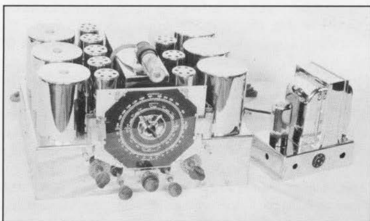
Figure 56. Super XII receiver and power supply. Late versions of the Super XII had a very small external power supply.
