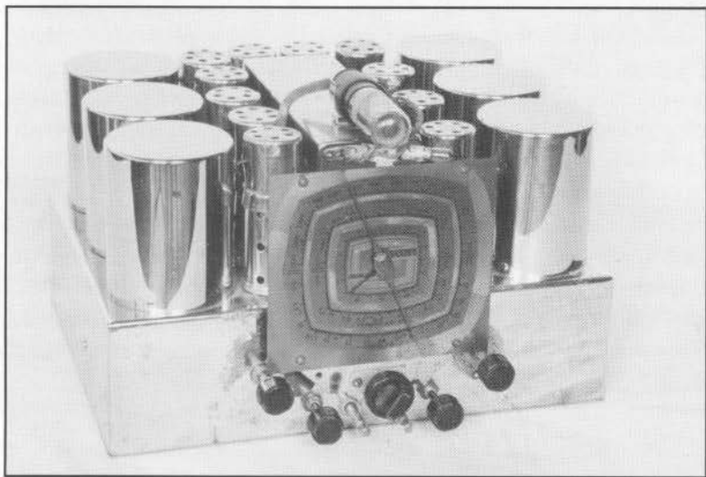
Figure 47. The Eighteen chassis. A rare variation of the Sixteen, with the phonograph scratch suppressor added.
