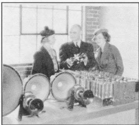
Figure 37. 40-Tube Quaranta receiver. The smallest of the famed receivers using tri-amplification.
