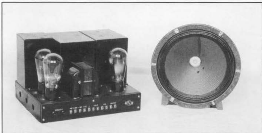
Figure 17. AC 10 power supply and speaker. Rola built the speaker, but has a Scott decal applied.
