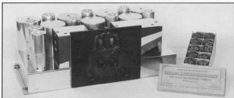
Figure 23. Allwave tuner and coil set. The first chrome chassis from Scott. The tube shields and coil covers are brushed aluminum, however.
