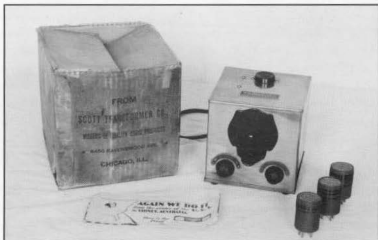
Figure 18. Short-wave converter and coils. There are two variations of the converter, one with a 4-prong connector for dc sets, and one with 5 prongs for ac sets.
