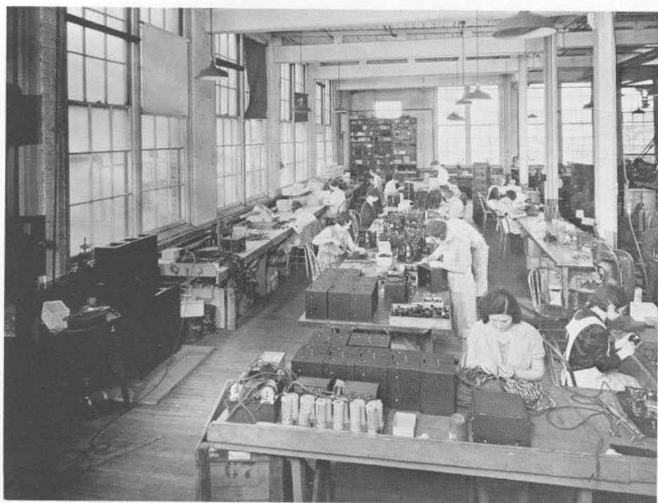
Fig. 7. An interior view of the National Company, in the early '30s, showing assembly of SW-3 receivers. Photo Credit: James Millen
