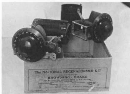
Fig. 5. The National Regenaformer Kit for home construction of the Browning-Drake receiver. The company address is given as 110 Brookline St., Cambridge, Mass. List price was $22.00.
