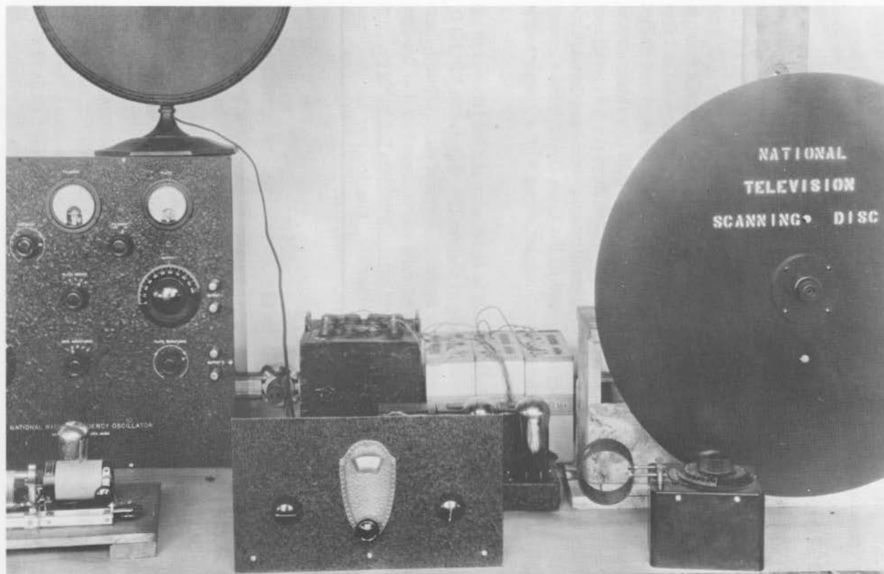
Fig. 9. Early television experiments at National, about 1927. Shown is a National SW-2 with TV scanning disc. In the background is a National RF oscillator and a Western Electric 540 A.W. speaker.
