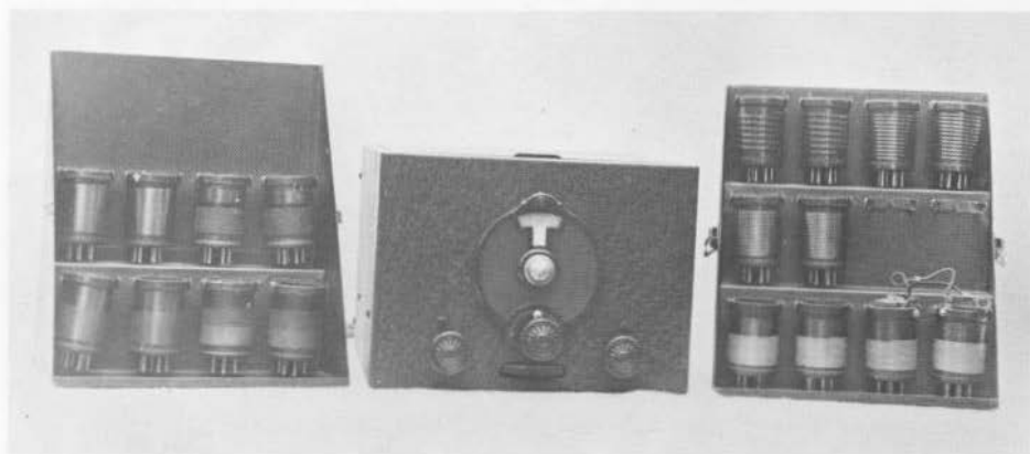
Fig. 8. The famous SW-3 receiver, with a set of coils in the NCC-10 National Coil Cabinet.
