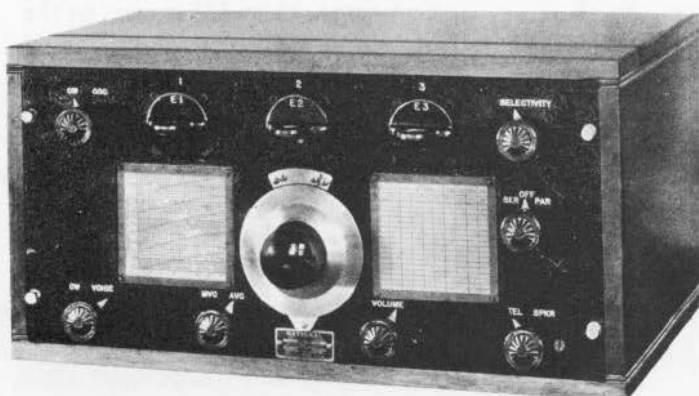
Fig. 10. The 1932 AGS-X in a custom walnut cabinet for table mounting. The Lamb type mechanical quartz filter provided single-signal operation. Another version, the AGU, had the three coils assembled into a single unit for ease of handling.
