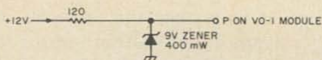
Fig. 2. Simple zener regulator improves transceiver stability greatly when battery supply starts to become "soft" after several hours use.
