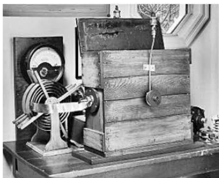
Maxim spark transmitter—"Old Betsy."
