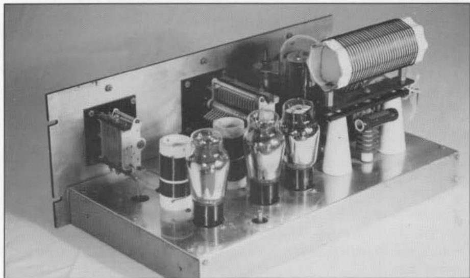
Figure 13. The Collins 4A transmitter. This was Collins' first and last try at the "low price" amateur transmitter market. Introduced in mid-1933 with a selling price around $60, less coils and tubes, it had 20 watts of CW output on 160/80/40 meter bands. (Author's collection...photo by author.)
