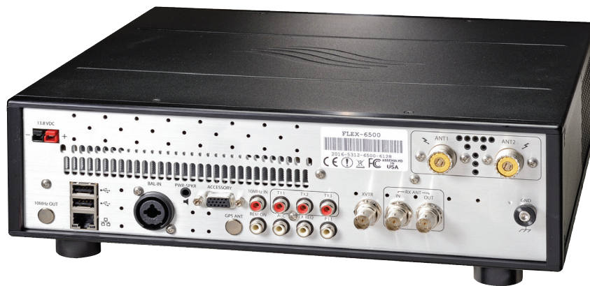
Figure 5 — The FLEX-6500 rear panel. Connections include two antenna jacks, transverter, receive antenna, powered speaker, 10 MHz reference input, three TR relay outputs for controlling power amplifiers and other external devices, balanced audio input, amplifier ALC, PTT, transmit interlock, Ethernet, and USB ports for SmartSDR functions. The 15-pin ACCESSORY jack has connections for audio line in/out, CW and FSK keying, PTT, and other features.
