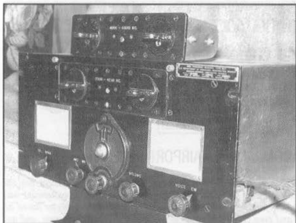
The National Co.'s 1933 RHP airport receiver. Note the long name plate, type BX dial and extra coil set. (All photos and drawings accompanying this column courtesy William Fizette.)
