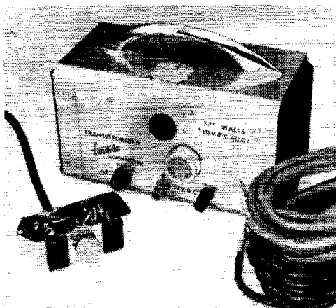
The Terado 300 watt inverter. The frequency control reed is visible between the 12-volt d.c. input terminals on the main unit. Cables at the right of the photograph are for connections to the battery and to the control unit at the left. The control unit, which can be mounted at a remote location, houses the output receptacle, voltage selector switch and indicator lamp. Although they are partially hidden in this photograph, cooling fins for the transistors are at each end of the main unit.
