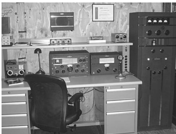
A complete Collins 30K station graces this shack. Directly behind the chair is the 75A1 receiver with matching speaker on the wall above. To the right of the receiver is the 310A exciter. The 30K-1 transmitter stands next to the desk.
