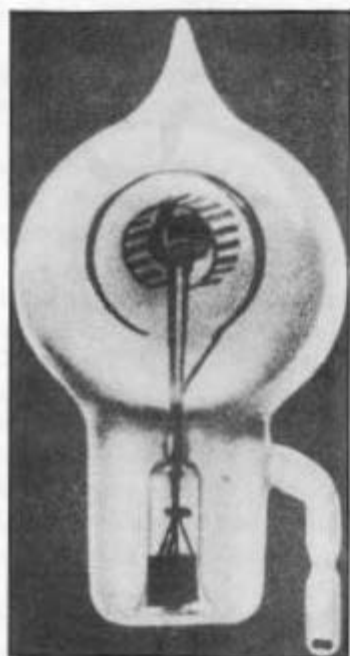
Fig. 3. Evolution to 1910: a gaseous device with the beam controlled electrostatically. (Adapted from DRP Nr. 249,142.)
