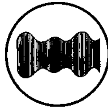
FIG. 6 R12, R15, AND L2 PROPERLY ADJUSTED, CARRIER BALANCE POTENTIOMETERS IMPROPERLY ADJUSTED
