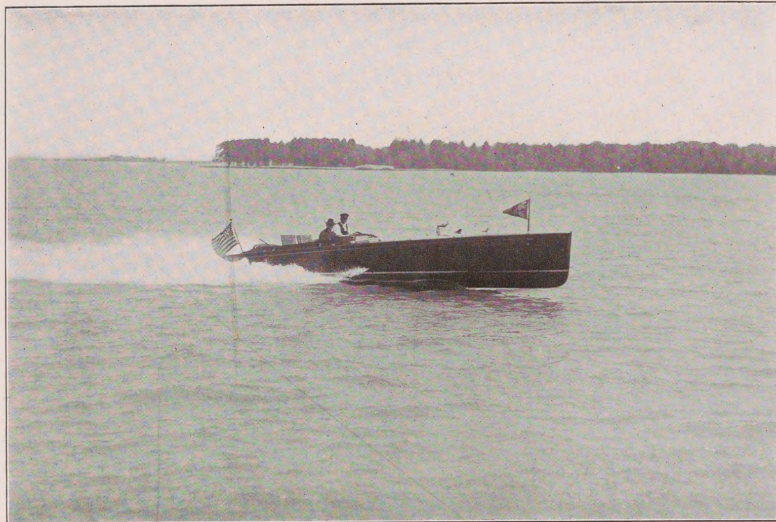
"Roamer," of Detroit, is owned by E. Holley and brother (the well-known makers of carburetors). This is our standard thirty footer with six-cylinder Van Blerck, electrically started. They consider the speed quite a sensation and averaged 35.6 m. p. h. up and down stream, with five men aboard.
