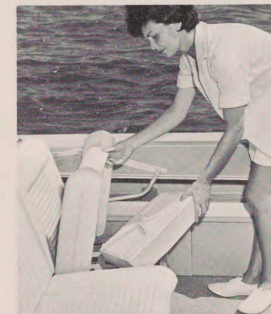
A Coast Guard-approved life preserver is an integral part of each seat, can be lifted out instantly in case of need.
