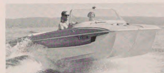
Tripod effect of sponsons and aft planing surface give Johnson boats the ability to zigzag across a wake like this with ease.
