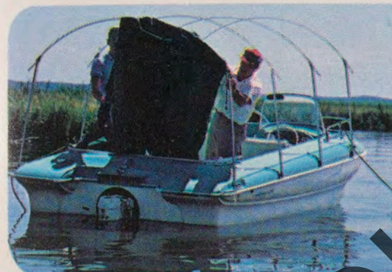
"Raising the roof" is a snap (or two) with Seasport's camper top, even while afloat. First, the sturdy anodized aluminum frame is installed, then the green and white canvas.
