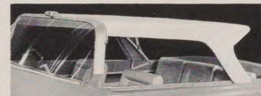
Convertible top snaps on or off with dual windshield latches. Waterproof 27-ounce fabric is non-shrinking, mildew-proof.
